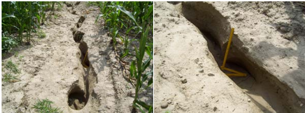
Figure 35: Pixendorf–chnozem: rill erosion (details) at the experimental field during corn crop.
