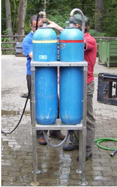
Figure 7: Deionization of the rain simulation water through clearing up tanks (left) and control of its electrical conductivity (right).
