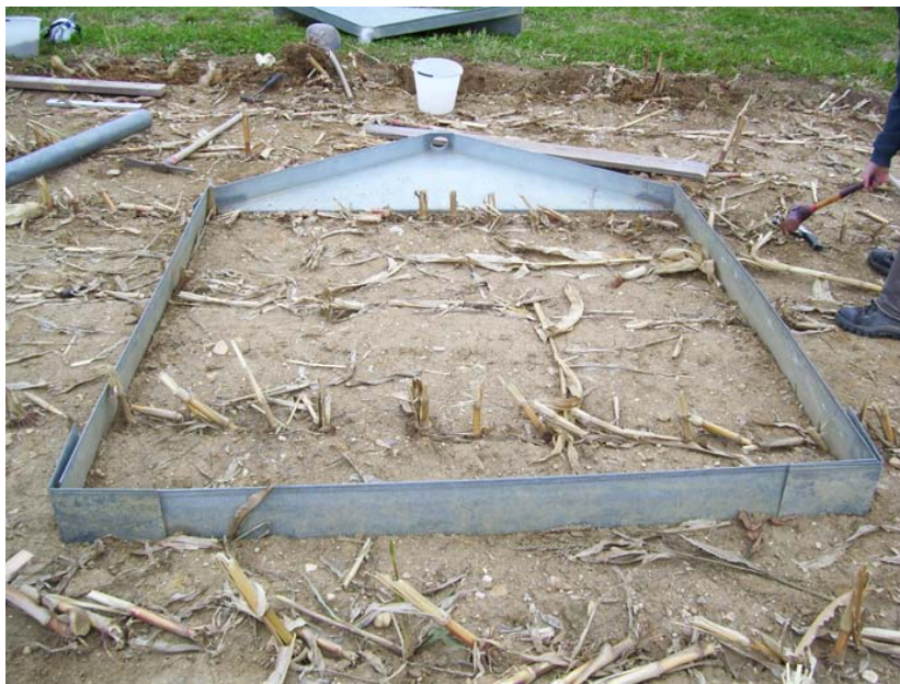
Figure 4: Installation of the 2m x 2m rain simulation plot.
