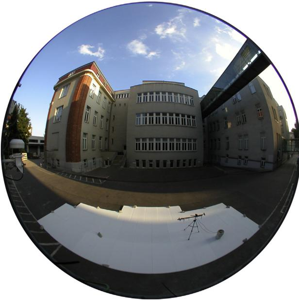
Fig. 3. View of south-facing PV modules taken with a camera with a fish-eye lens. The placement of the white Styrofoam panels in front of the PV modules is shown.
