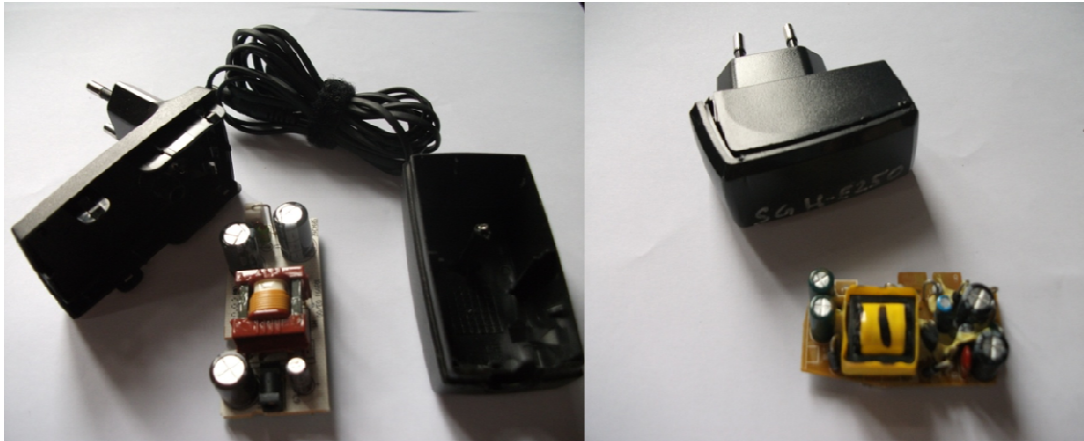
Figure 26: Sample of dismantling trials: Switched mode mobile phone battery charger, part 3
