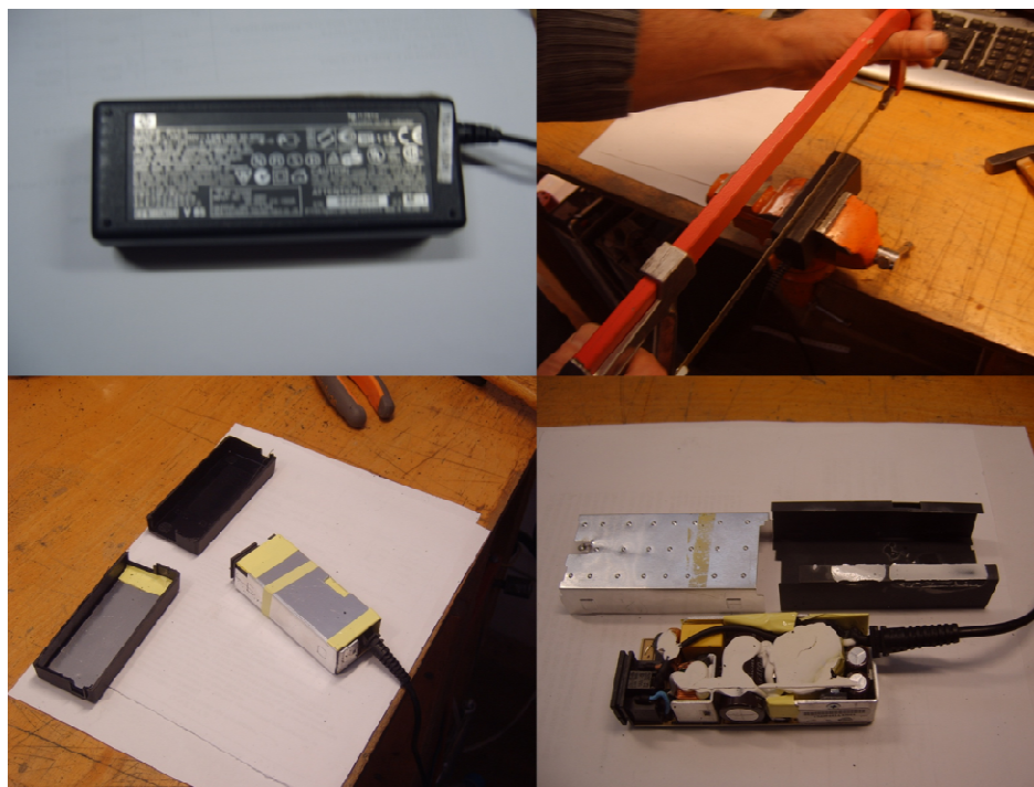
Figure 22: Sample of dismantling trials: Switched-mode notebook EPS, part 1
