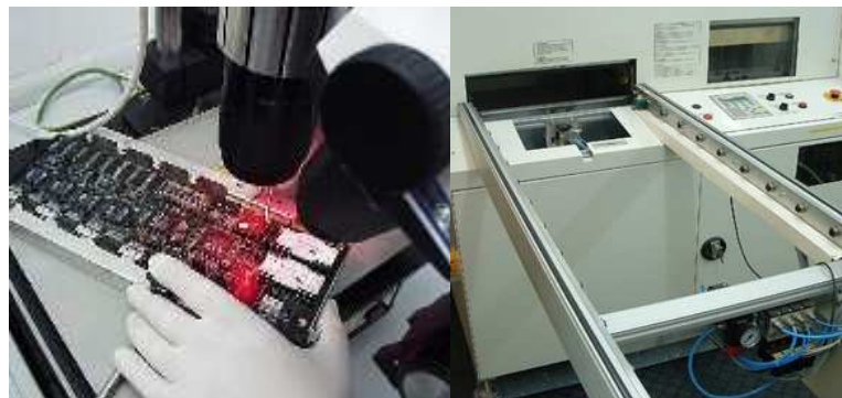
Figure 42: Desoldering techniques for BGA components – infrared radiation (left) and vapor (right) (source: DCE, 2012)
