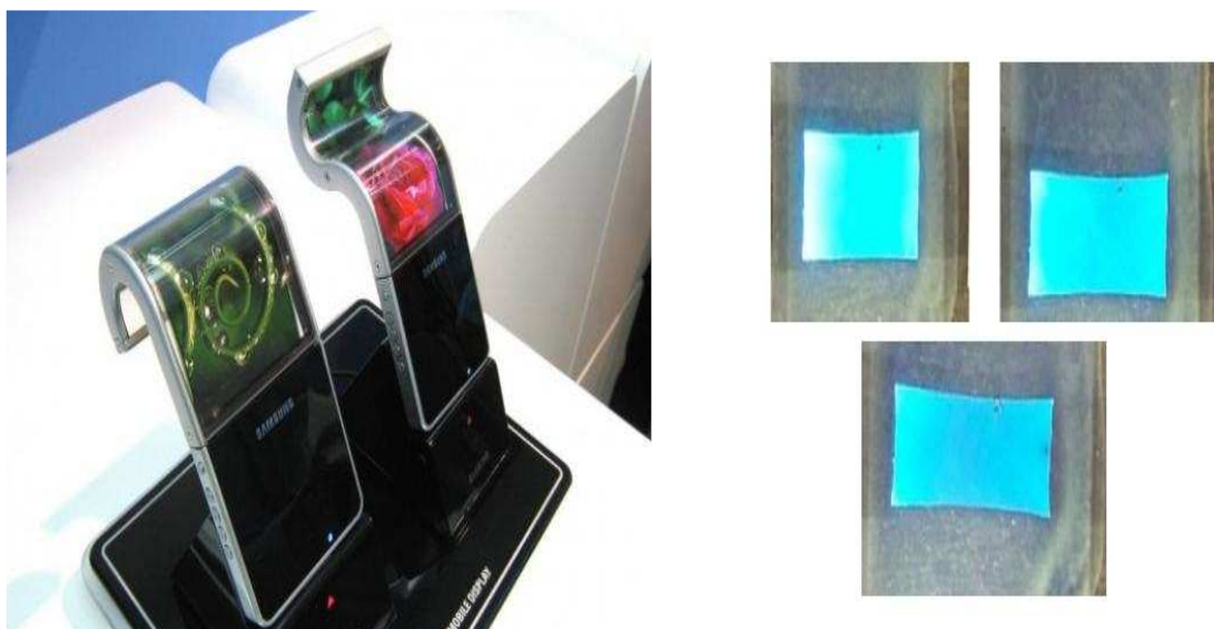
Figure 16: Bendable AMOLED (left) and stretchable AMOLED (right) (source: PHONEARENA, 2011, GIZMAG, 2012)
