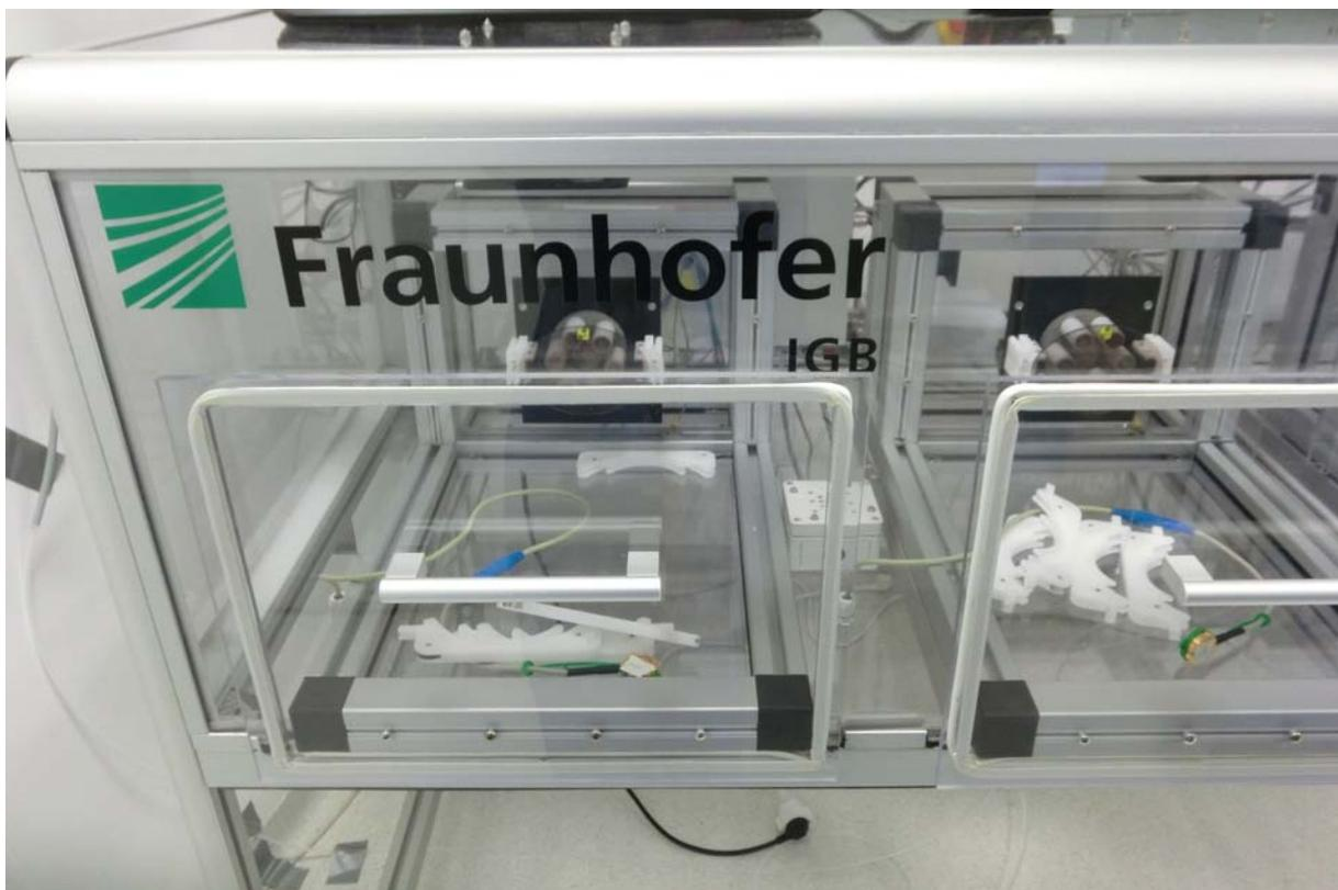
**Figure 4.23:** IT-3a cell culture incubator table (Fraunhofer IGB)
