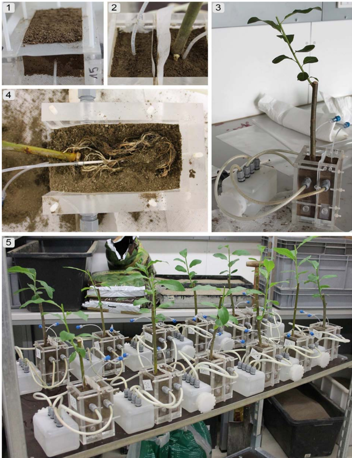
Figure 3: Photographs of the rhizobox assembly: (1) bulk soil and 2-mm rhizosphere compartment; (4) willow planting and installation of Rhizon sampler; (2) detailed view of final rhizobox - bulk soil, rhizosphere and root compartment including Rhizon samplers; (3) rhizobox at start of the experiment including watering system; (5) replicates for all treatments before setting up the experiment in the greenhouse.
