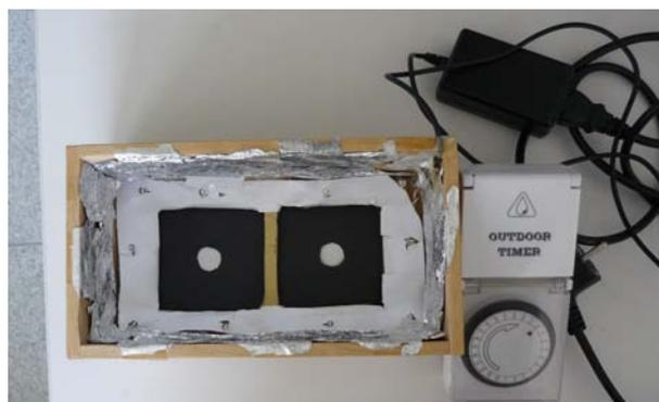
Figure 4.2: Wooden box with 10 LEDs in parallel mode was placed above fungal cultures in plant tissue culture boxes. The light was switched on for fixed time intervals, additionally the box prevented from uncontrolled influences from light because it was covered with black paper on top.
