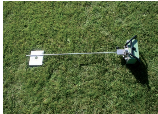
Abb. 19: Penetrollogger der Firma EIJKELKAMP AG-RESEARCH EQUIPMENT
