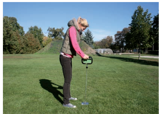
Abb. 20: Penetrollogger in Gebrauch
