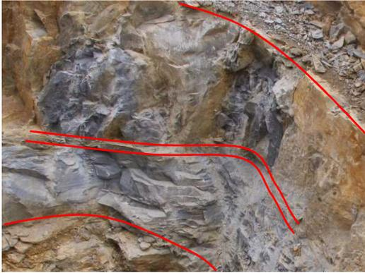
Layer 6 is a grey 95 cm thick layer, similar to layer 4 and 2. The fracture plane appears smooth like a wood plate- The scratch hardness reaches 5. The measurements with the Schmidt hammer display a higher strength of 59.5 MPa.
