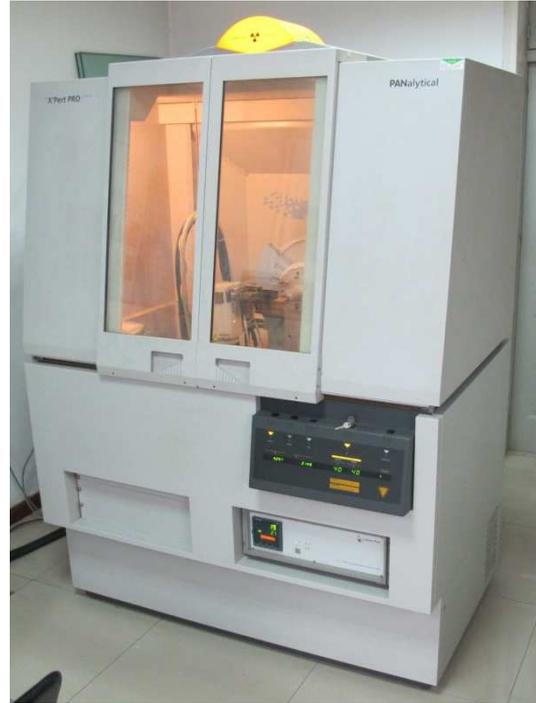
Figure 42: X-Ray Diffractometer of China University of Geoscience (Photo: Mayrhofer 2013)
