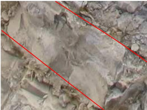
A 27 cm thick grey layer is similar to layer 2 but a bit darker grey coloured. It also displays a slow HCl reaction. The scratch hardness of 4 and the slightly rough fracture plane indicates similar properties like layer 2. Just the measured strength is with 52.5 MPa a bit higher.
