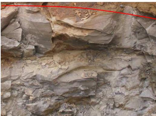
The following layer is grey coloured. Similar to the aforementioned grey layer but the scratch hardness reaches just 4. Here the measurements with the Schmidt hammer show strength of 36.2 MPa. It is the last possible layer to assess.
