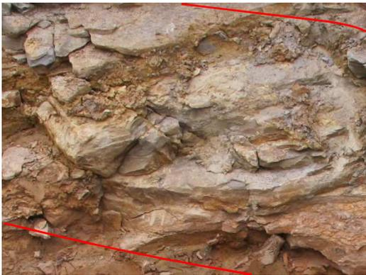
Layer 9 is a reddish, 60 cm thick layer of mudstone. With strength of 14.4 MPa it has a weak appearance as also the scratch hardness is only 1. It is interposed with cracks and loose rock topples out. The HCl test displays a slow reaction. The fracture plane appears from soft to slightly rough.
