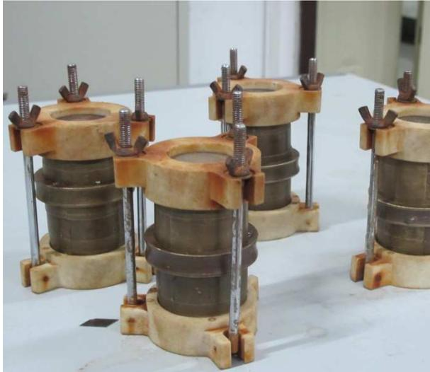
Figure 32: Prepared sample for triaxial test (Photo: Mayrhofer 2012)
