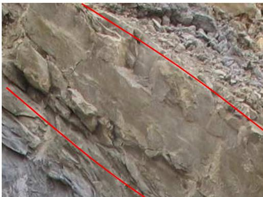
The first layer of the Artificial opening is a brown- grey coloured marlstone with a scratch hardness of 1-2. The total dimension is 0.4 m. The fracture plane appears rough. Smith hammer measurements show strength of 41 MPa. The transmission zone of layer 1 and 2 is undisturbed.
