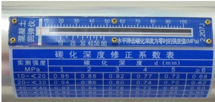
Figure 30: Readout scale of the Schmidt hammer (Photo: Mayrhofer 2012)
