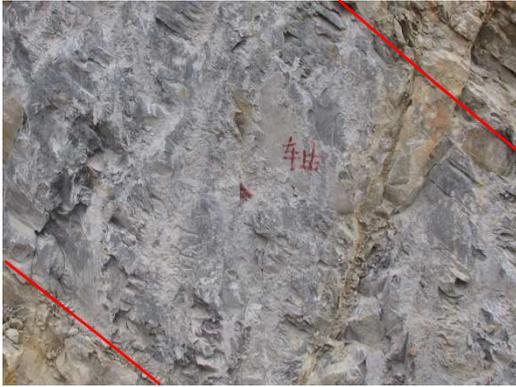
This grey interbedding has a dimension of 1.7 m. The fracture plane is between smooth and slightly rough. A slight reaction of HCl shows a medium carbonate content. The scratch hardness reaches 4 with a measured strength of 52.7 MPa.
