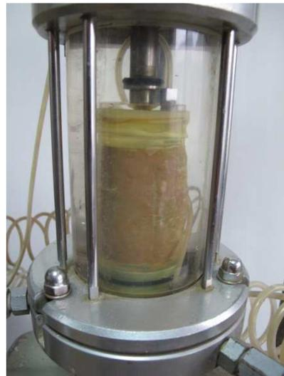
Figure 34: Sheared sample at an axial strain of 15% (Photo: Mayrhofer 2012)
