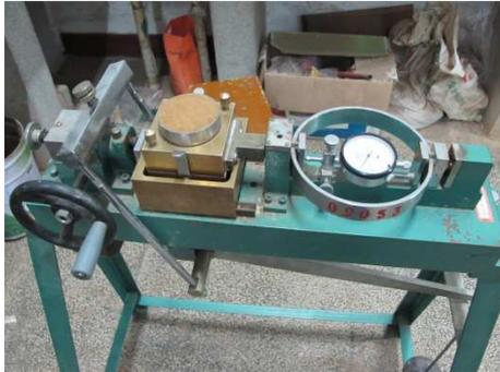
Figure 35: Device for quick shear test (Photo: Mayrhofer 2012)
