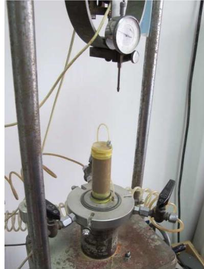
Figure 33: Fixed sample on the triaxial device (Photo: Mayrhofer 2012)
