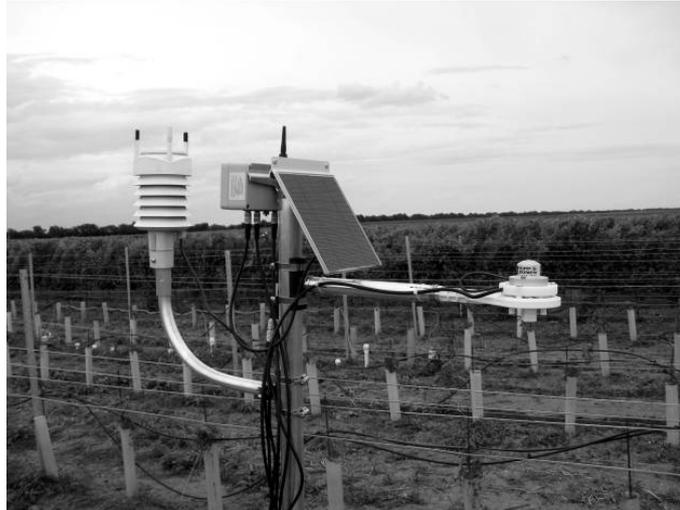
Fig. 8.1: Measuring station with RTU, solar panel and weather instruments (photo: R. Nolz)
