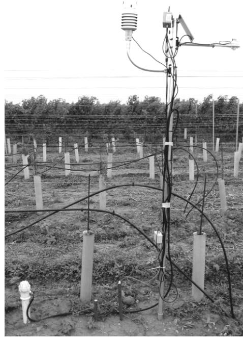
**Figure 9.1: Measuring station with RTU, solar panel, weather sensors, FDR-probe (white cap) and three watermark sensors in 10, 30 and 50 cm depth.**
