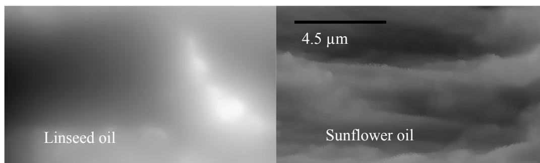
Fig. 2. Two AFM images (topography images) of linseed oil- and sunflower oil-coated Typha fibers
