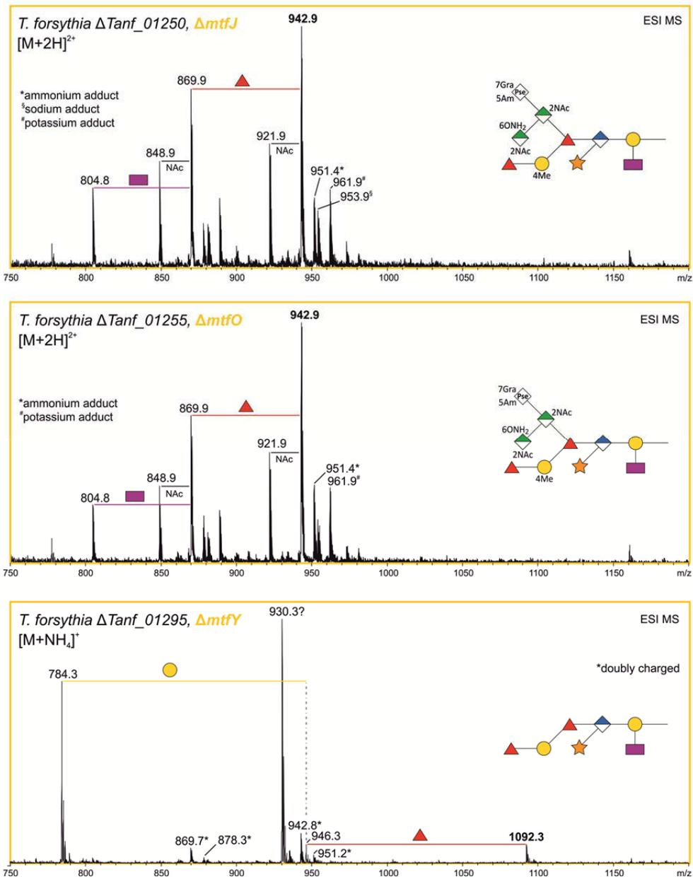
**Figure 8** Deconvoluted ESI-IT MS sum spectra of  $\beta$ -eliminated TfSb O-glycans from three *T. forsythia* ATCC 43037 methyltransferase knock-out mutants. The glycan structure of the highest mass peak (written in bold) is shown as symbolic representation. Mass peaks from the subsequent fragmentation pattern were assigned according to the loss of carbohydrate units and modifications. Relative peak intensities of occurring peaks are given on the y axis (M.B. Tomek, unpublished data).
