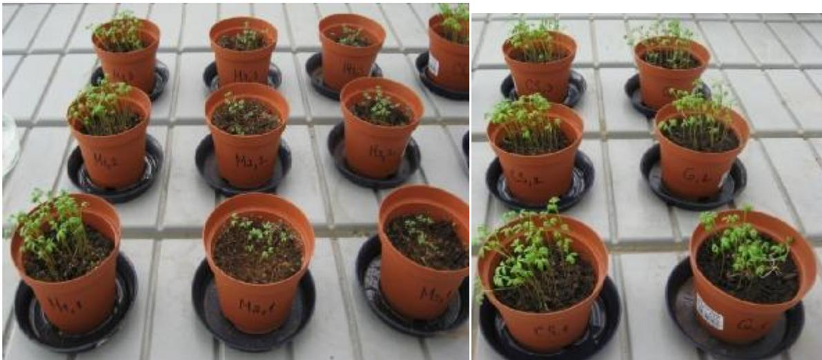
Figure 6: Cress test results (from left to the right: mix 1, mix 2, mix 3, commercial substrate and Grand substrate)
