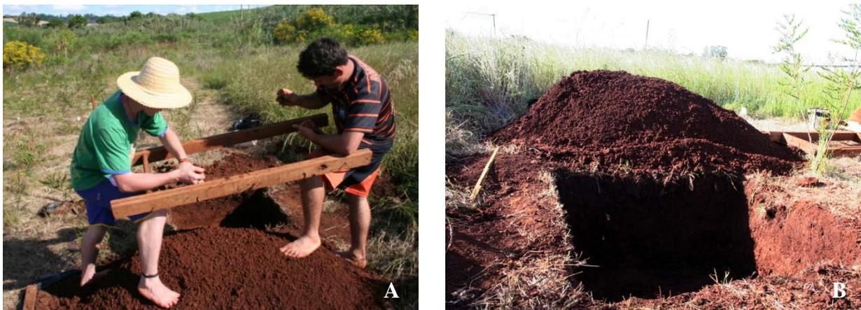
Figure 15: (A) Sieving the stripped earth in order to extract the roots that had remained in soil (B) Soil was excavated in an area of 1 m<sup>2</sup> and deep as 50 cm. Campus, UFSM – CESNORS, Frederico Wesphalen, 10.12.2012.
