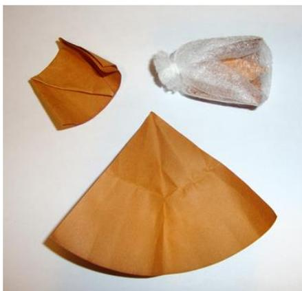
**Figure 1:** Preparation of the iron oxide impregnated filter papers: cut, folded and put into protection nets
