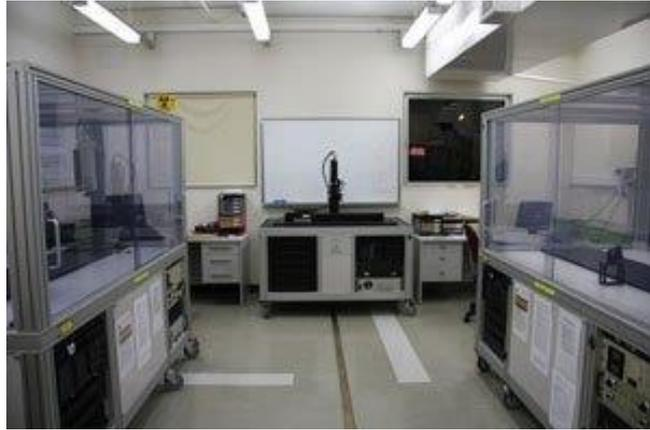
**Figure 14: The three measurement units of SilviScan-3. Left to right: the densitometer (density variation), cell scanner (tree ring orientations and cross-sectional cell dimensions) and diffractometer (microfibril angle, wood stiffness), which are integrated via a server. [Photo: ©Rob Evans, CSIRO]**
