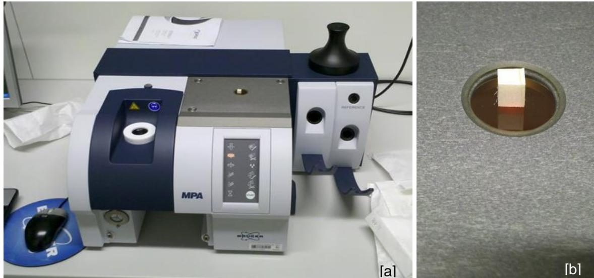
**Figure 12: [a] MPA; [b] Sample on an integrating sphere**
