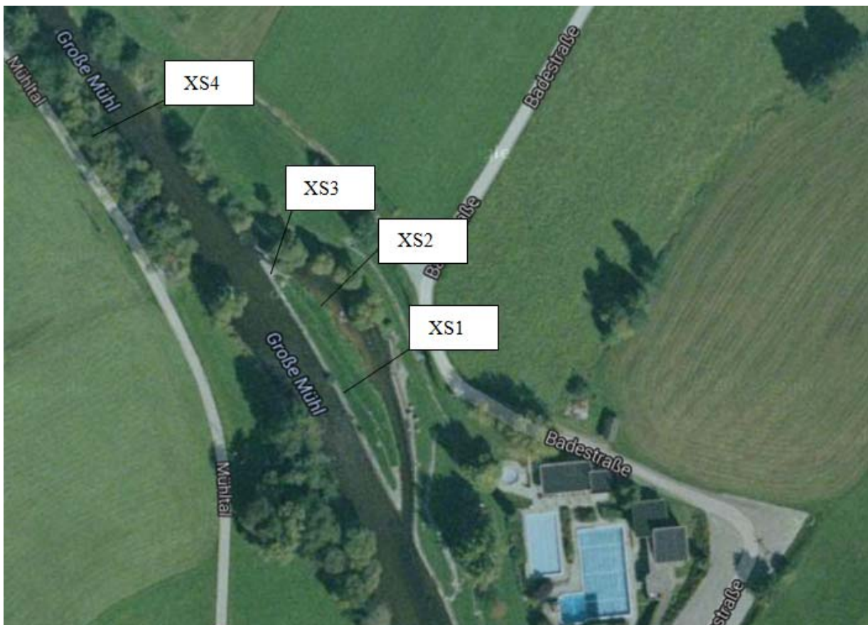
Figure 31 Cross sections of the on-site observations and discharge measures in October 2013 for the final calibration in HEC-RAS
