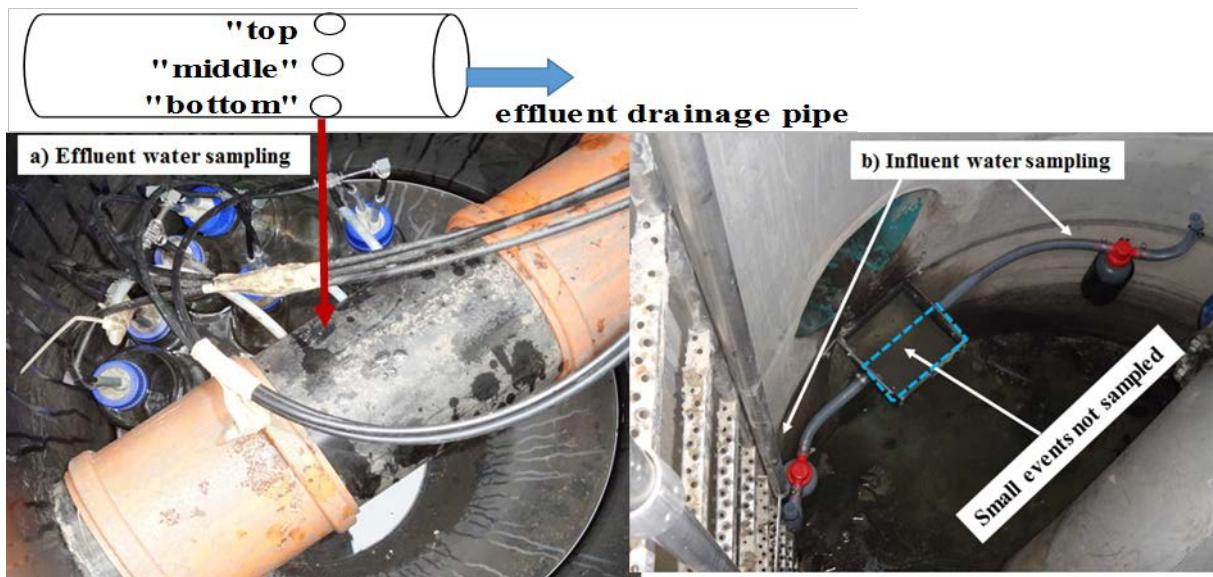
Figure 7. Passive sampling device of effluent (a) and influent (b) installed at GSA-L.
