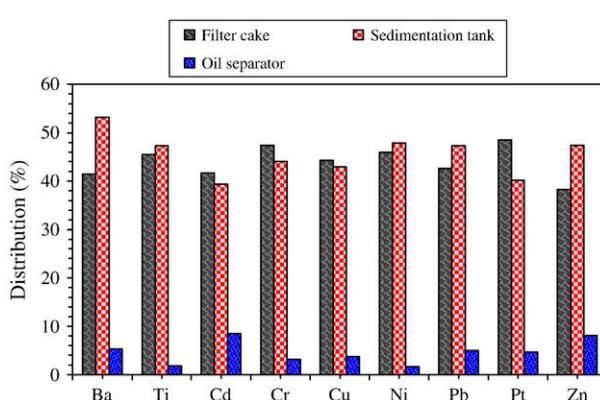
Fig. 5. Distribution of metal parameters removed in different sections of the treatment plant.
