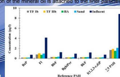
Fig. 6: PAH removal efficiency using real highway runoff
