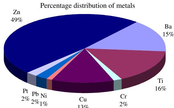
Fig. 6. Mass distribution of metals retained in filter cake (geotextile filter material), sedimentation tank and oil separator.
