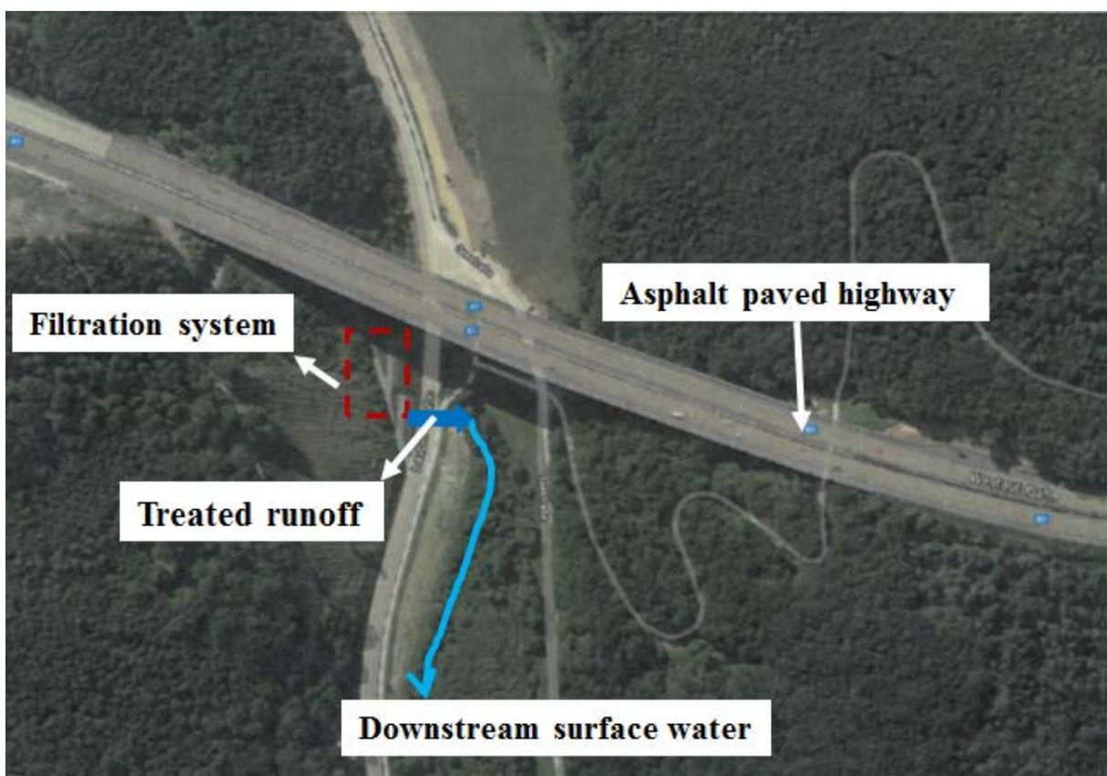
Figure 8. Picture of the non-urban highway catchment area. Dashed red line indicates the underground concrete vault filled with Aquafilt® (GSA-W), the treated highway runoff is discharged (Blue line) to the downstream surface water (light blue line).
