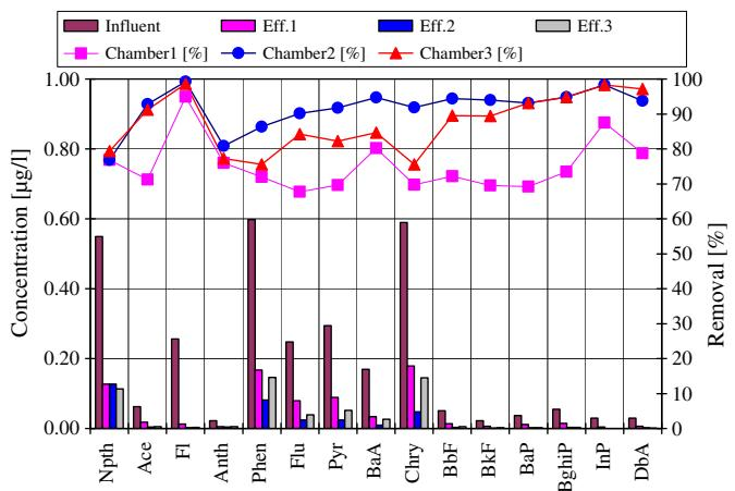
**Fig. 4.** Comparison of influent and effluent individual PAH mean concentrations and the calculated removal efficiency from each filter chamber.
