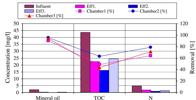
**Fig. 2.** Comparison of influent and effluent mineral oil, TOC and  $\text{NH}_4\text{-N}$  mean concentrations and their calculated removal efficiency from each filter chamber.
