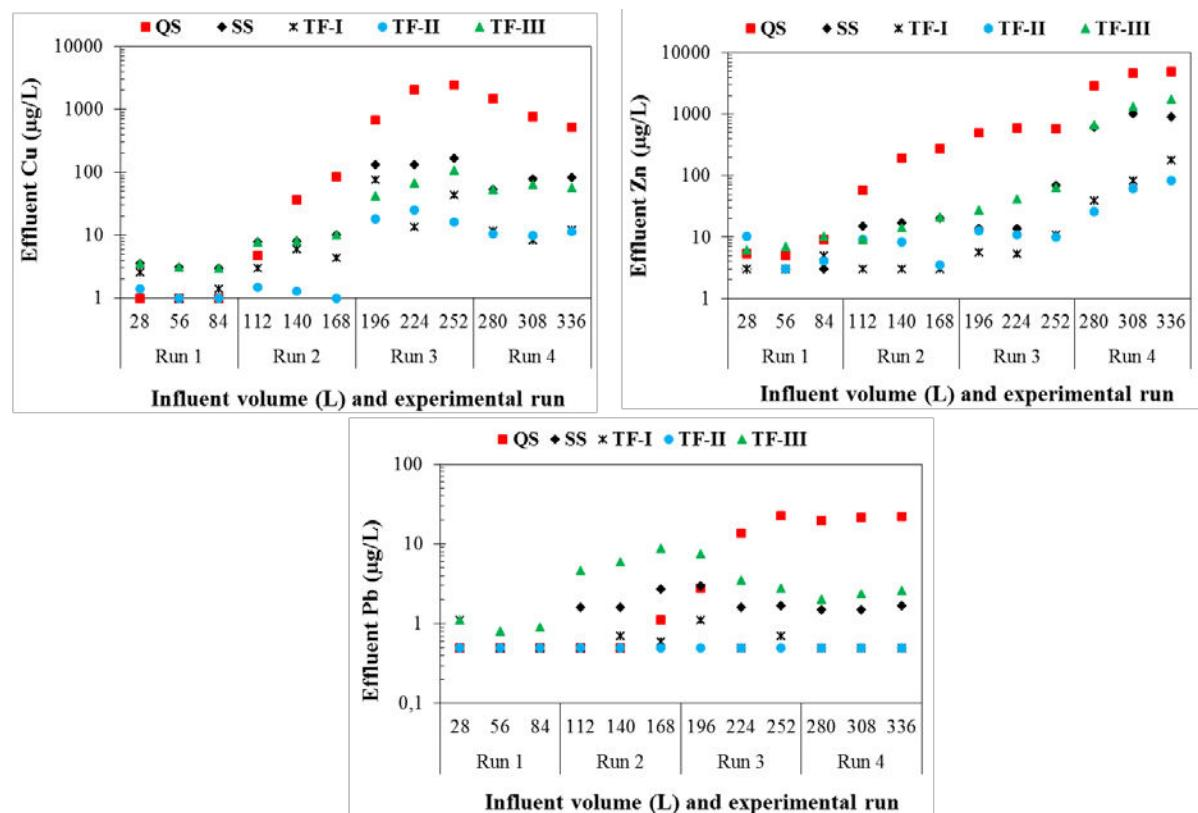
Figure 2. Effluent concentrations of heavy metals with different synthetic stormwater dosings (Run 1 – Run 4, see Table 2) under high hydraulic load experimental conditions as a function of treated volume.
