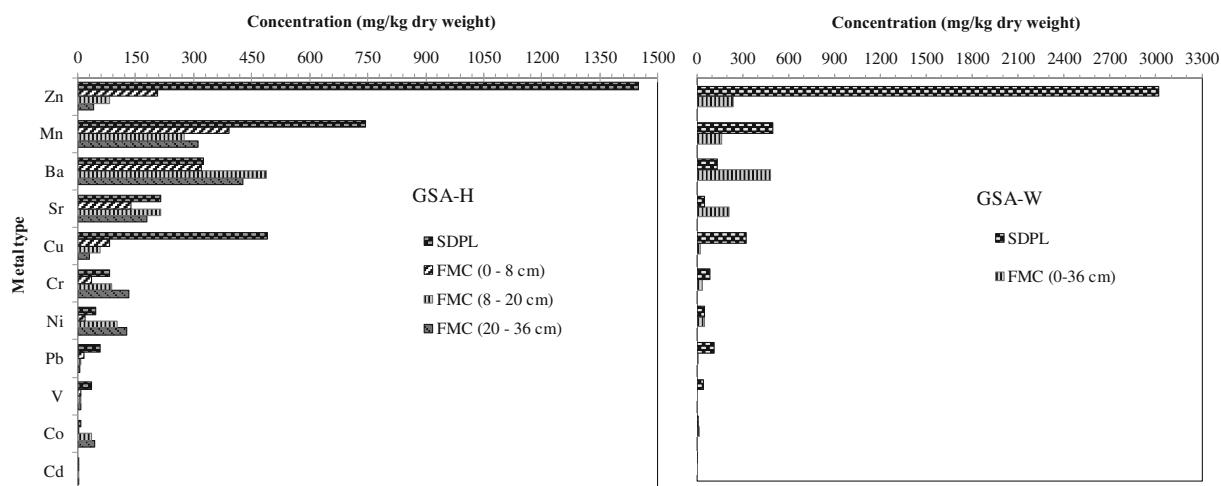
**Fig. 4** Profiles of heavy metals in SDPL and filter media layer collected from two media filtration treatment systems
