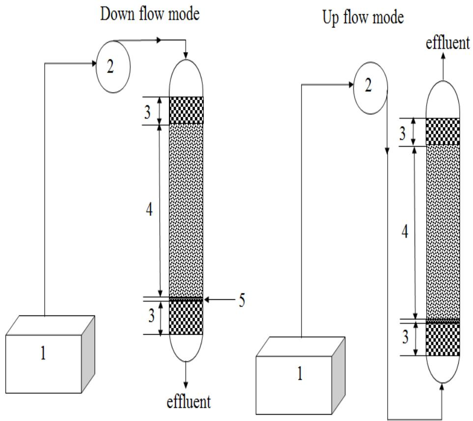
Figure 15. Schematic overview of the column setup to study effect of flow mode and heavy metal sorption capacity at filter media exhaustion. Schematic set-up for column breakthrough experiments: (1) influent feed solution; (2) peristaltic pump; (3) 40 mm glass beads; (4) fritted glass filter ; (5) 200 mm filter media bed; (6) effluent.
