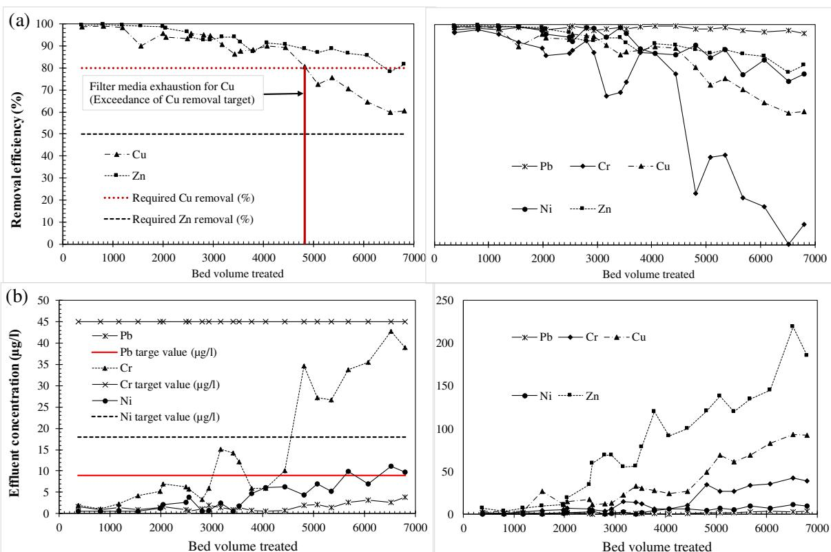
**Fig. 6** Removal efficiency (%) of heavy metals (a) and effluent concentrations (b) versus column flow through number of bed volumes (1 BV = 193 ml). The lines are not fitting functions; they connect points to facilitate visualization
