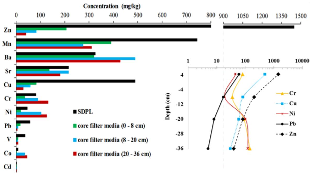
Figure 16. Profiles of heavy metals in surface deposited particle layer (SDPL) and core filter media collected from filtration system treating parking lot runoff (GSA-H).
