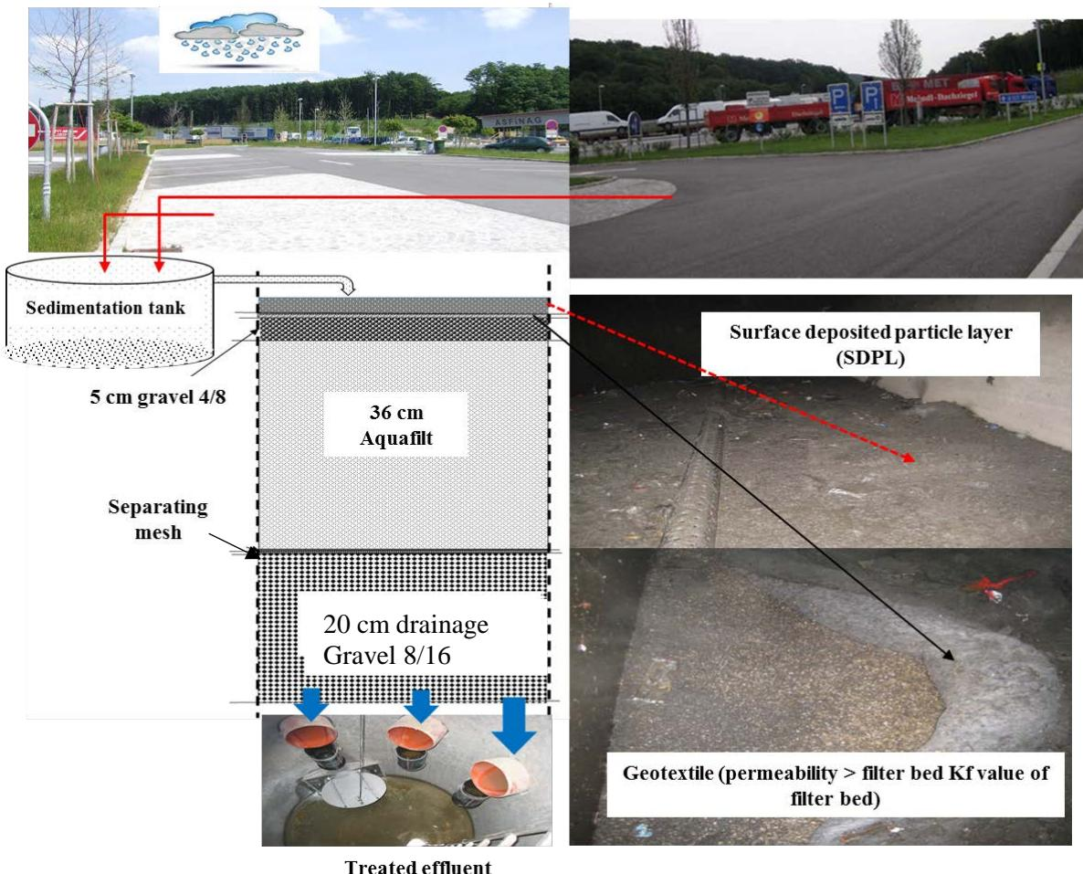
Figure 5. Picture of the parking lot at Hinterbrühl (top), layout of the filtration system, GSA-H (bottom left) and particle layer after 7 years of operation.
