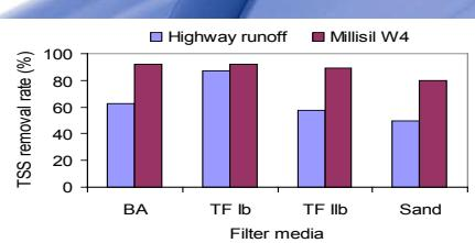
Fig. 5: Comparison of particle removal rate from real highway runoff and Millisil W4
