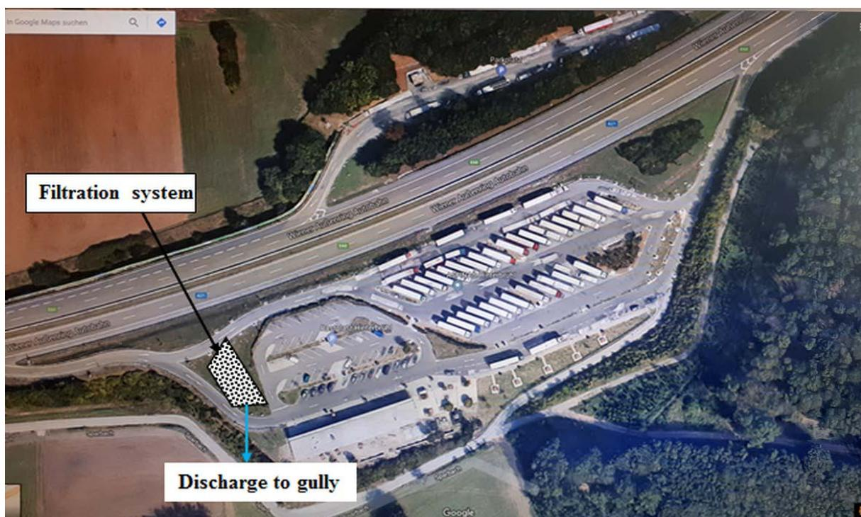
Figure 4. Overview of the parking lot and adjacent highway catchment area (GSA-H), installed filtration system and effluent drainage.
