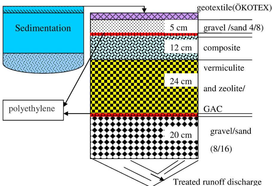
**Fig. 1.** A general set up of filtration treatment components with layered filter bed.
