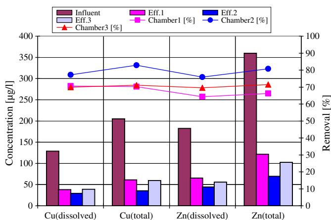
**Fig. 3.** Comparison of influent and effluent Cu and Zn mean concentrations and their calculated removal efficiency from each filter chamber.
