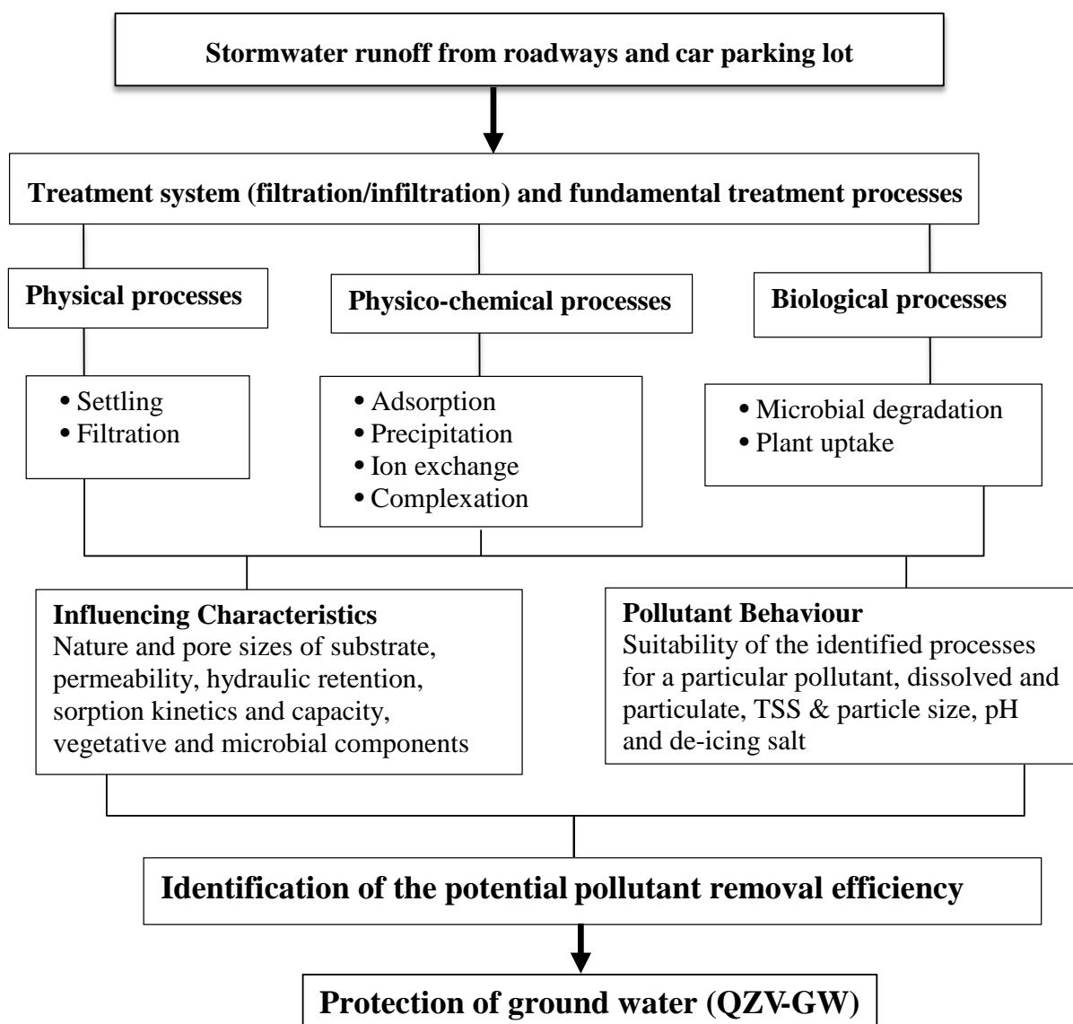
Figure 2. Fundamental unit processes in relation to BMP characteristics and pollutant behaviour (adopted and modified from Scholes et al., 2008).
