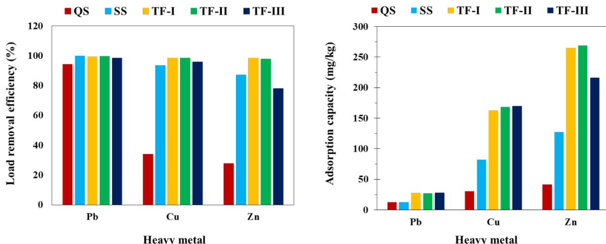
Figure 3. Overall removal efficiency (left) and adsorption capacity (right) of heavy metals by each filter media type.
