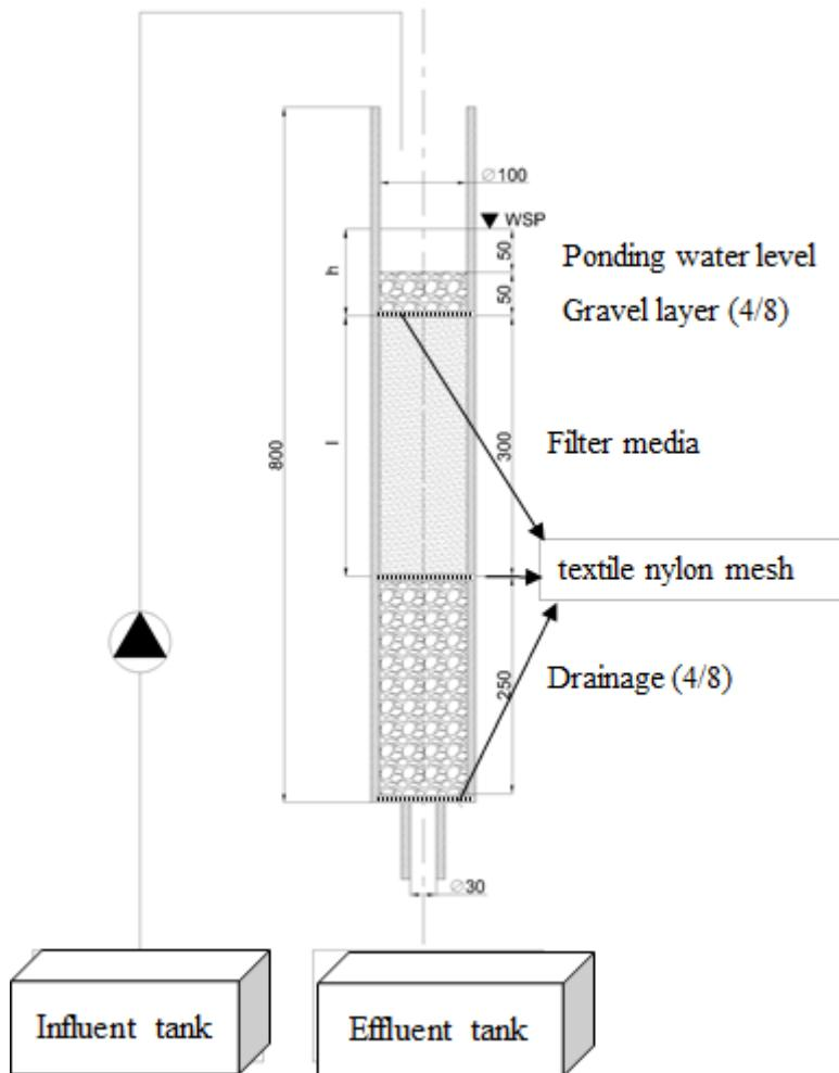
Figure 14. Schematic overview of the column setup to study the effect of hydraulic load on heavy metal removal. Subsequently, the filter media preloaded with heavy metals were flushed with 42 L of NaCl solution (5 g/L NaCl) to evaluate the remobilization of heavy metals.
