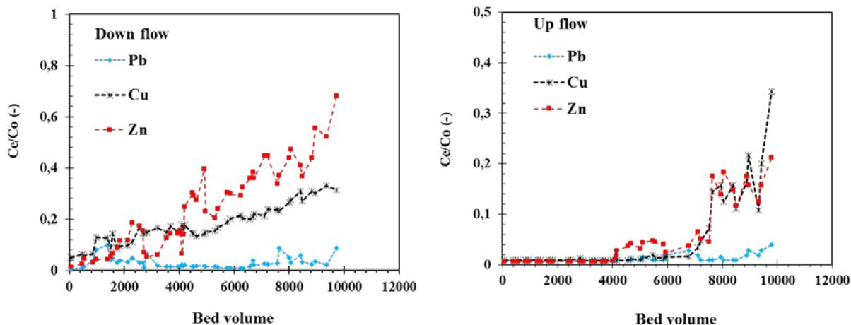
Figure 4. Comparison of breakthrough curves of Cu, Pb and Zn in downflow and upflow mode as a function of bed volume at a volumetric flow rate of 50 mL/min (50% of its maximum saturated flow rate) and filter bed volume of 160 mL. Note that to facilitate visibility of the graph, the Y-axis is different in each case.
