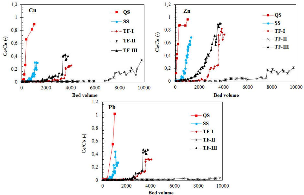
Figure 5. Breakthrough curves of column experiments for metal mixtures. The lines are not fitting functions; they simply connect points to facilitate visualization.
