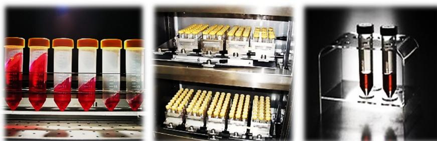
**Figure 36:** DisposableTubeSpin<sup>®</sup> bioreactor 50 with orbitally rotating shaker consists of a sterile PITFE- filter, which is permeable to gas and has a working volume from 1 ml to 35 ml. 10 ml was the working volume in this experiment (taken from (6)).
