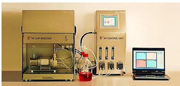
**Figure 44:** Z<sup>®</sup>RP 2000 H bioreactor system with control unit and breeder (taken from (11)).
