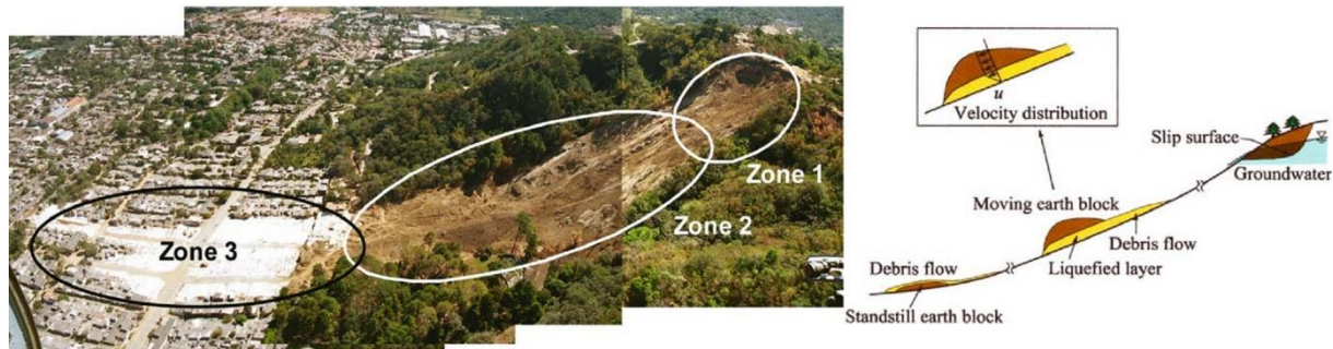
Figure 10: DF zonation (Zone 1 = initiation zone, zone 2 = transition zone, zone 3 = deposition zone), and an illustrative example of the development of a DF (Konagai et al., 2007; Takahashi, 2007).
