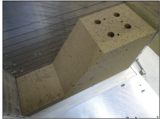
Fig. 87: Soil after centrifuge
