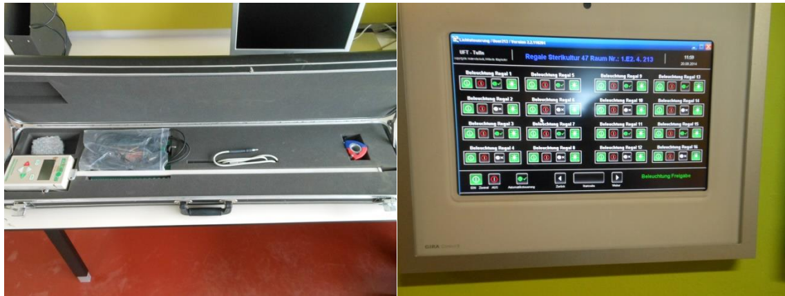
Figure 17: Left side: SPAD LP-80; first measurement of light conditions; Right side: Automatic light control system (GIRA Control 9) of growth chambers
