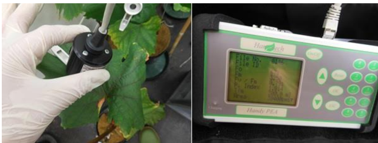
Figure 23: Handy PEA chlorophyll fluorometer at the measurement on June 5 th ; left side: sensor unit and leafclips; right side: control unit.
