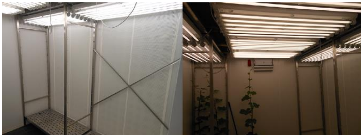
Figure 22: Both pitures taken on May 11 th ; Left side: Rearrangement of light modules to the top of the chamber; Right side: Equal distribution of light modules
