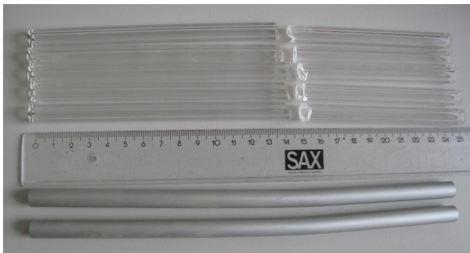
Fig. 4.13 Broken piles after the tests. Left side is the pile head. The breakage of acrylic piles and the plastic hinge in aluminium piles occurred at about 14 cm measured from left (about 1 cm below the slip surface).
