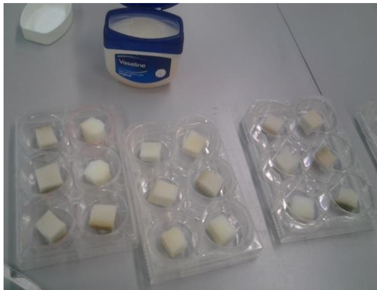
Figure 2.4: Foam cuboids fixed with petroleum jelly in cylindrical compartments inside plastic cartridges.
