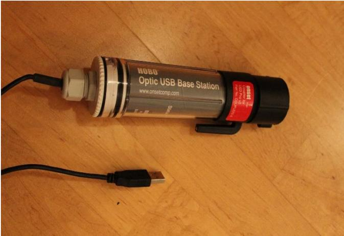
Abbildung 3.2: Onset HOBO Optic USB Base Station
