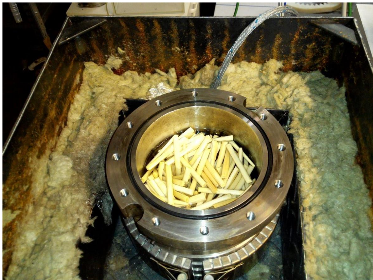
Figure 6. Opened tubular HTC reactor filled with bamboo sticks and water.
