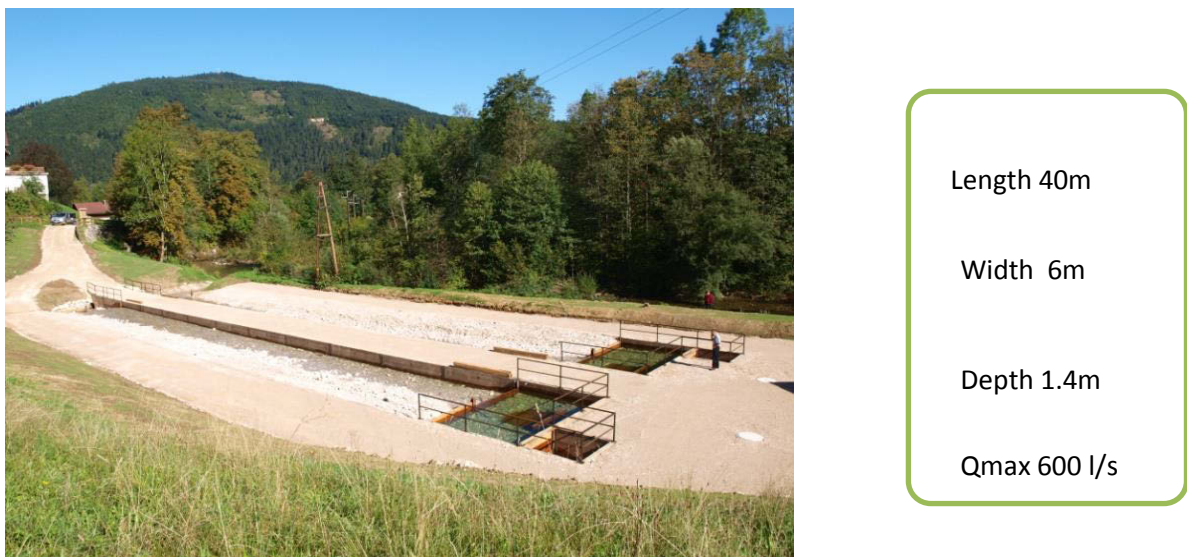
Figure 10. HyTEC experimental channels (Auer, 2011)
