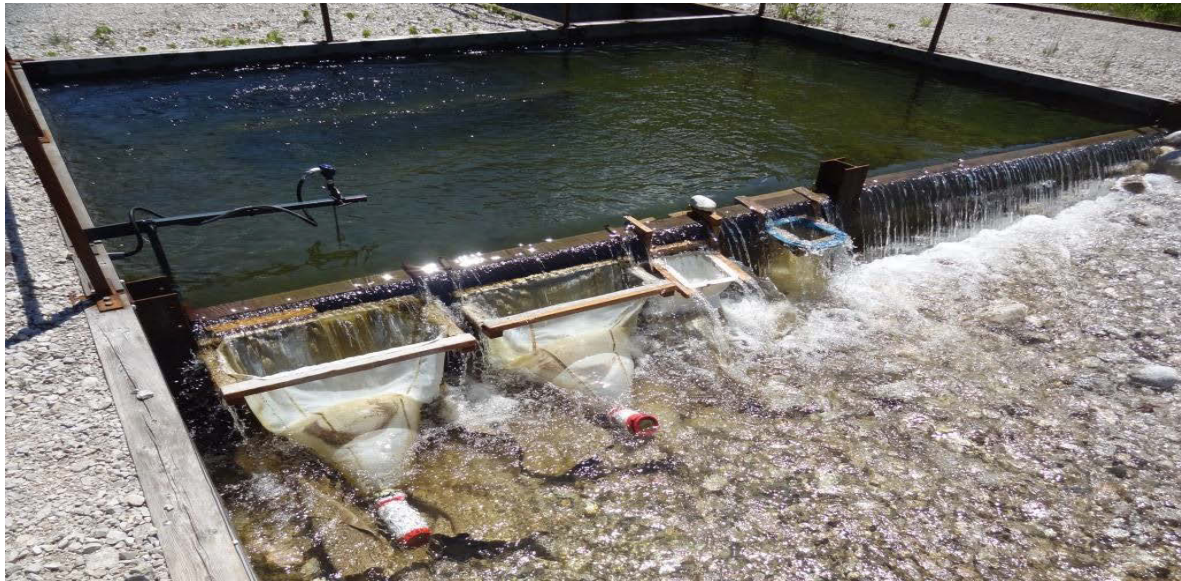
Figure 18. Mixing basin with plankton nets for collection of zoo- and phytoplankton (Fischer, 2013)
