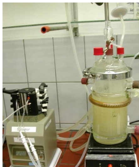
Figure 3: Fermenter setup - on the right the glass fermenter on the magnetic stirrer, on the left the pump which pushes the air into fermenter
