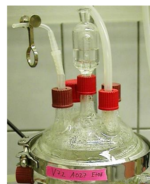
Figure 4: Lid of a fermenter with the fermentation lock in the middle, sampling tube with clamp on the left and tube for the air input on the
