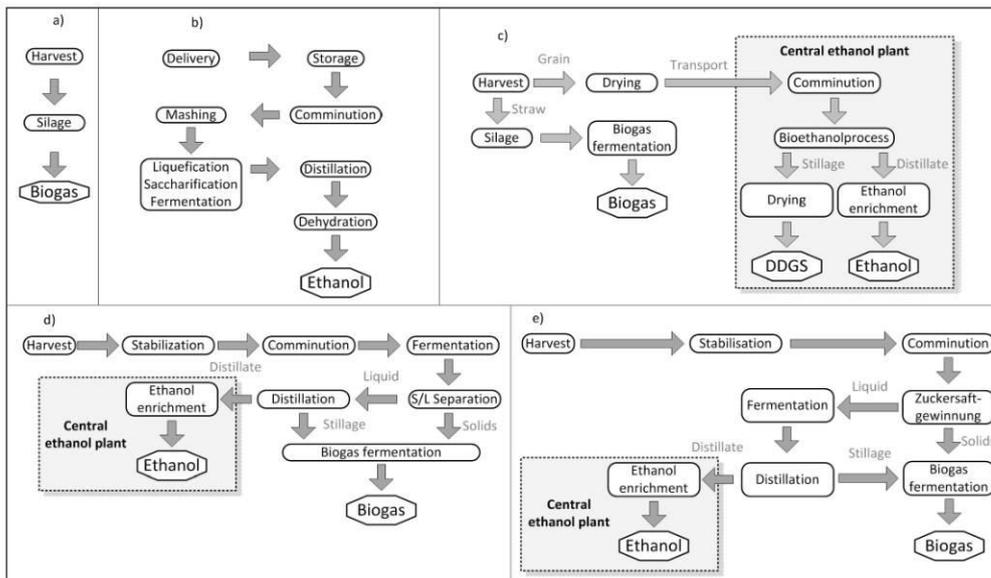
Figure 2: Evaluated process concepts: a) Benchmark Biogas variant, b) Benchmark Ethanol variant, c) Grain sorghum variant with separate grain and straw utilization, d) Sweet sorghum variant with whole plant fermentation, e) Sweet sorghum variant with separate juice fermentation
