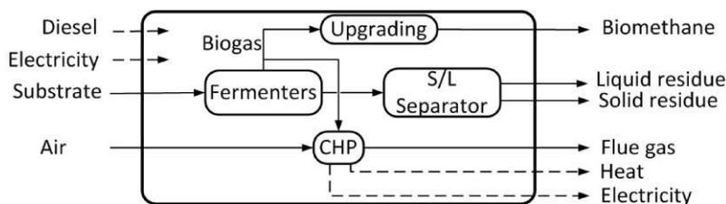
Figure 1: Flow sheet of the monitored biogas plant
