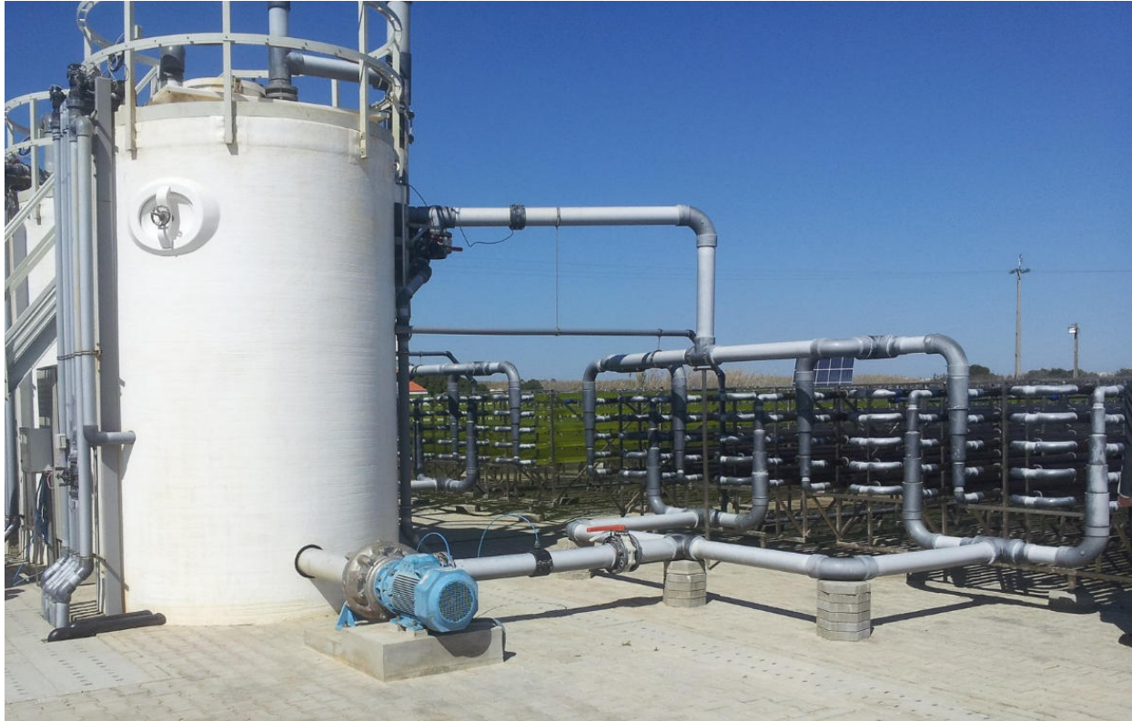
Figure 8: Tubular photobioreactor at Necton S.A., Olhao, Portugal. The manifolds to split the tubes can be seen on the right side. The white tower for degassing and cooling can be seen on the left side. Photograph taken by the author in April 2016.
