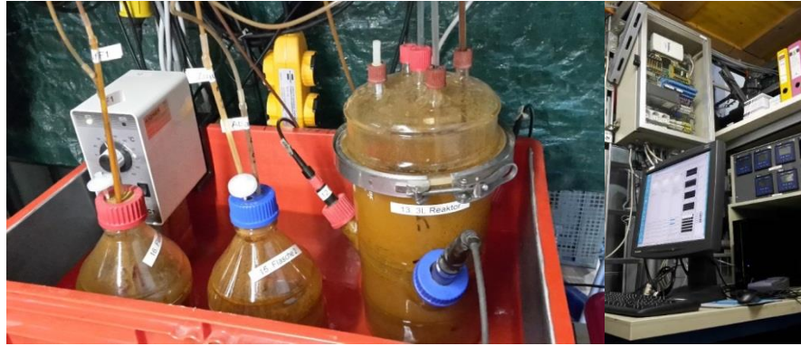
Figure 14: 3L PNA reactor set up at the technical hall of the Institute.
