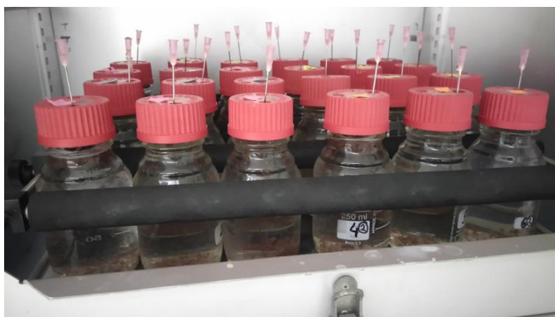
Figure 13: Set up of the 24 batch flasks in the incubator. All flasks were equipped with needles to release pressure and to be able to draw samples with a syringe.
