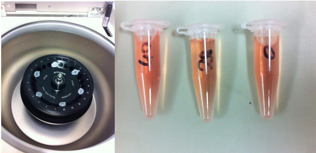
Figure 34: View into the centrifuge (left), eppis with standards from 40% [v/v] to 0% DMSO after centrifugation.
