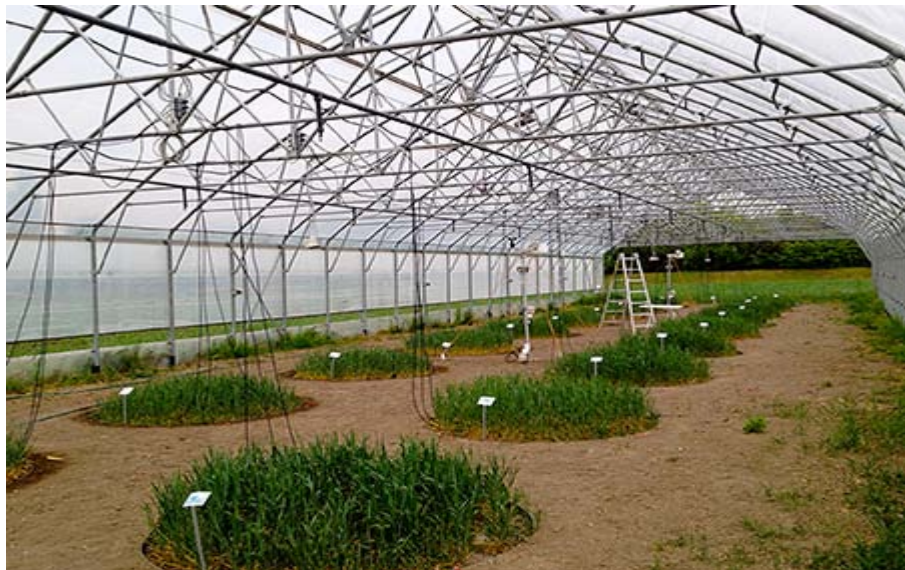
Figure 4.1: Experimental winter wheat plots containing three different soil types (calcaric phaeozem, calcic chernozem, gleyic phaeozem) subjected to long-time and prognosticated rainfall variations according to regionalized climate change models.
