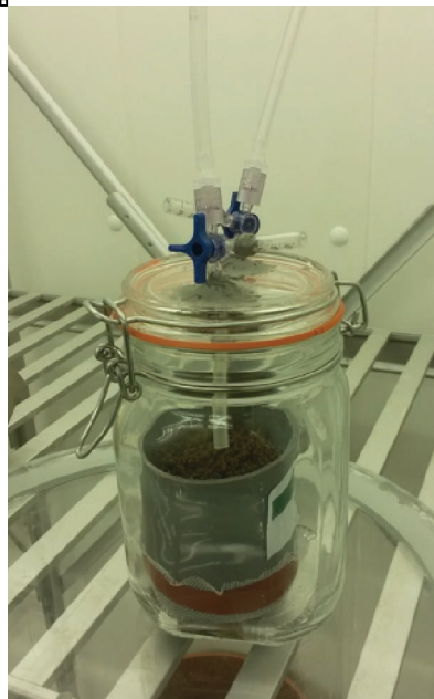
Figure 6. LGR measurement system for N 2 O determination
