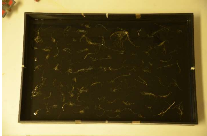
Figure 7: Black tray for estimating the sample size and the generation of sub-samples
