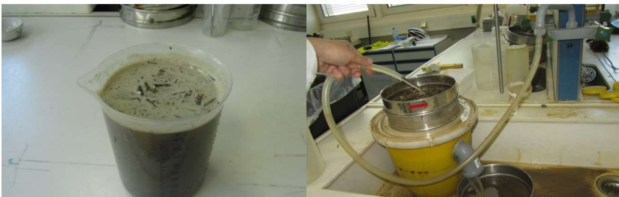
Figure 5: Left: Suspension including the dissolved soil sample. Right: Sieving using a water hose.
