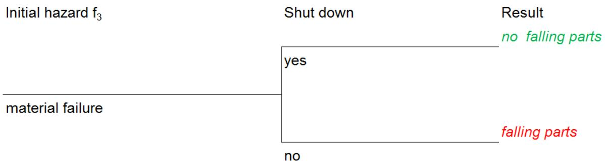
Figure 5.4: Event-tree with the initial hazard material failure (own figure)
