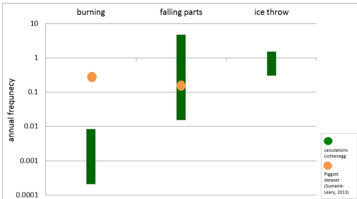
Figure 6.1: Occurrence frequency bandwidths of the three unwanted events calculated by PSA for the example SWT in Lichtenegg (green) and observed failure frequencies of the Piggott dataset (orange) (own figure)
