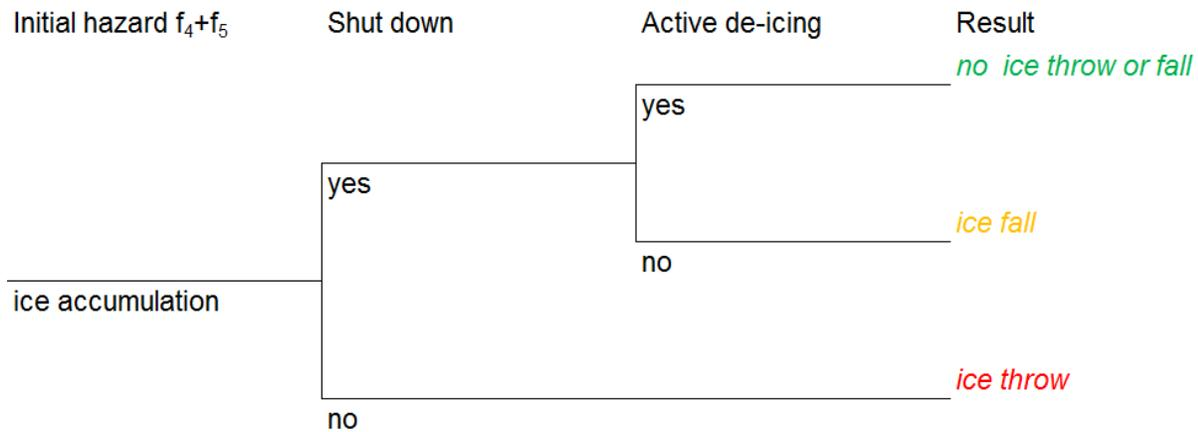
Figure 5.5: Event-tree with the initial hazard ice accumulation (own figure)
