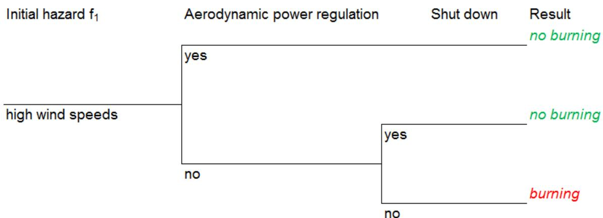
Figure 5.2: Event-tree with the initial hazard high wind speeds (own figure)
