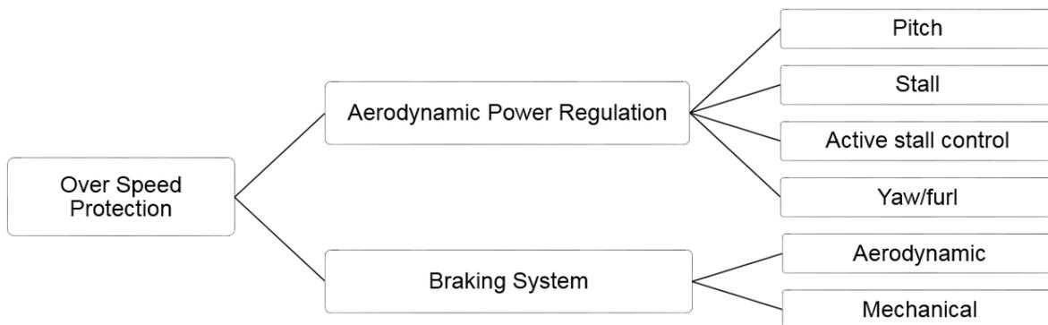
Figure 2.9: Most common overspeed protection systems of wind turbines (own figure)
