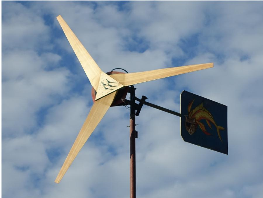
Figure 2.7: Self-constructed SWT referring to Piggott's design built in Germany, 2016 (picture by KanTe)
