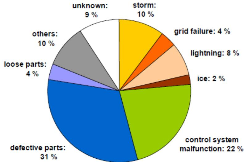
Figure 4.3: Causes for failure of 235 SWT in the WMEP 1990 to 2007 (Kühn, 2007)
