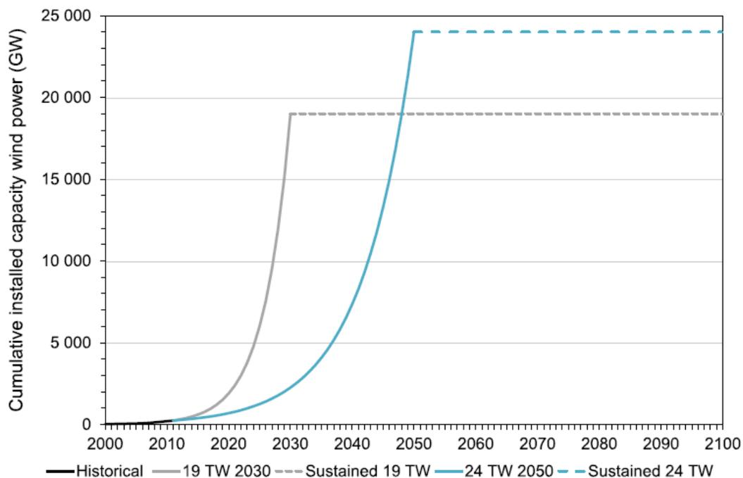
Figure 1.1: Cumulative installed capacity of wind energy described by a logistic curve fitted to historical data reaching 24 TW by 2050 (Davidsson *et al.*, 2014)
