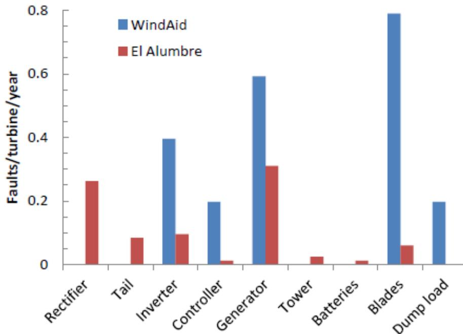
Figure 4.1: Normalized comparison of the breakdown of faults per component of Piggott SWT experienced by the development organizations WindAid and Soluciones Prácticas in Peru (Sumanik-Leary, 2013).
