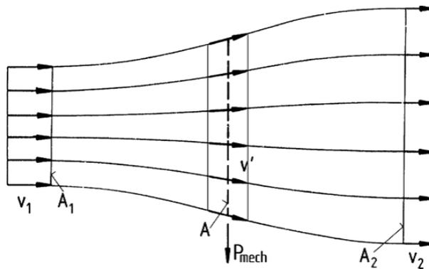
Figure 2.2: Relation of velocity and area of wind in front of, at and behind the turbine (Hau, 2014)
