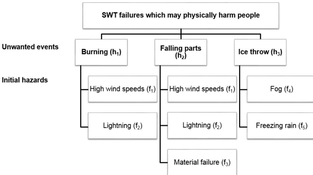
Figure 4.4: SWT failures which may physically harm people with their occurrence frequencies  $h_j$  and the initial hazards causing them with their occurrence frequency  $f_i$  (own figure)
