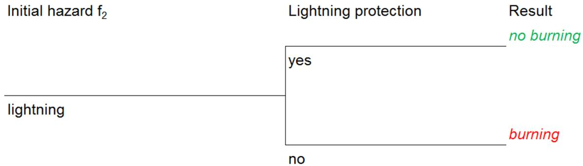
Figure 5.3: Event-tree with the initial hazard lightning (own figure)
