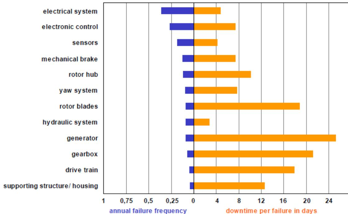
Figure 4.2: Frequency of failure by main components and related downtime for 235 SWT in the WMEP 1990 to 2007 (Kühn, 2007)
