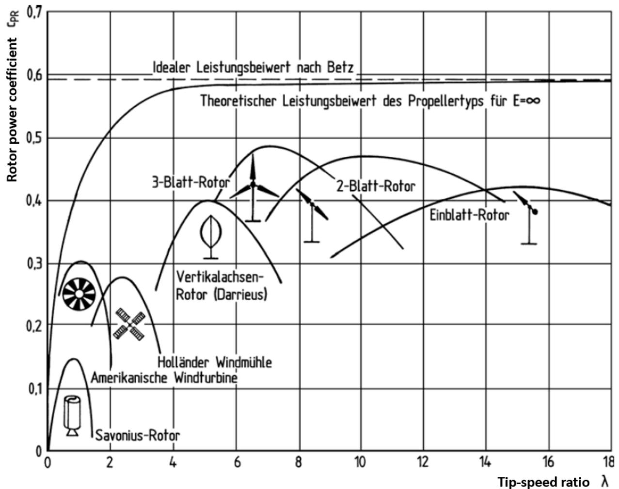
Figure 2.6: Tip-speed ratio and power coefficient of different turbine designs (Hau, 2014)
