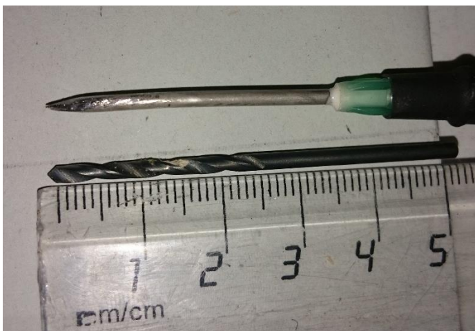
Figure 14: Close-up of applied Granier-type sap flow sensor and drillers for perforating tree stems.
