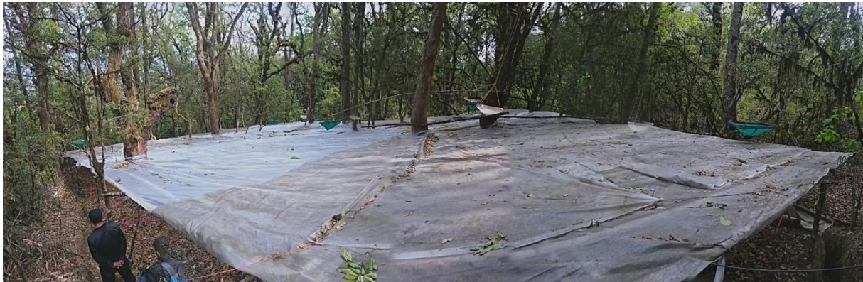
Figure 8: Roof with plastic foil at the broadleaf forest site, Bhutan/Wangdue Phodrang district.
