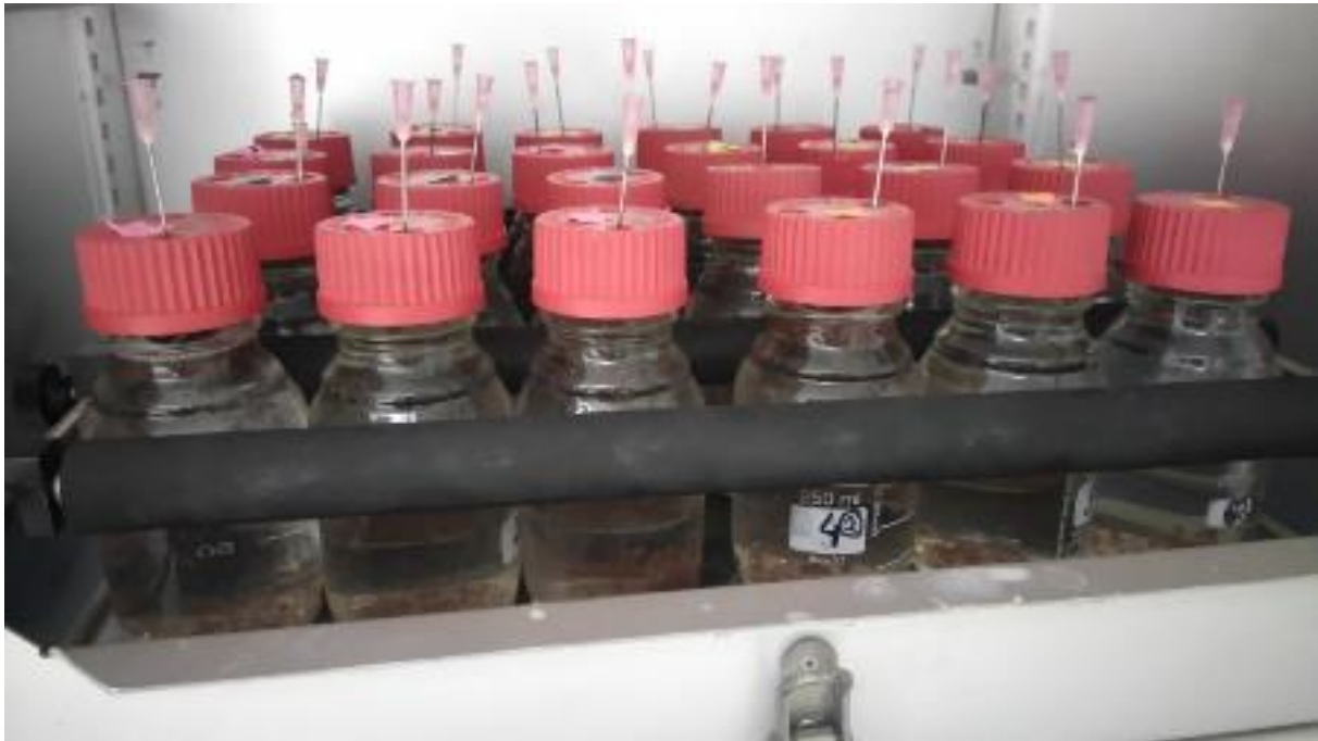
Figure 4: Batch test setup (Schitzenhofer 2016)
