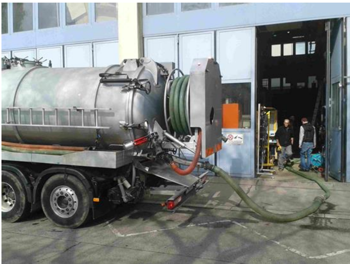
Figure 13: Takeover of reject water at the pilot plant station (Weissenbacher et al. 2017).
