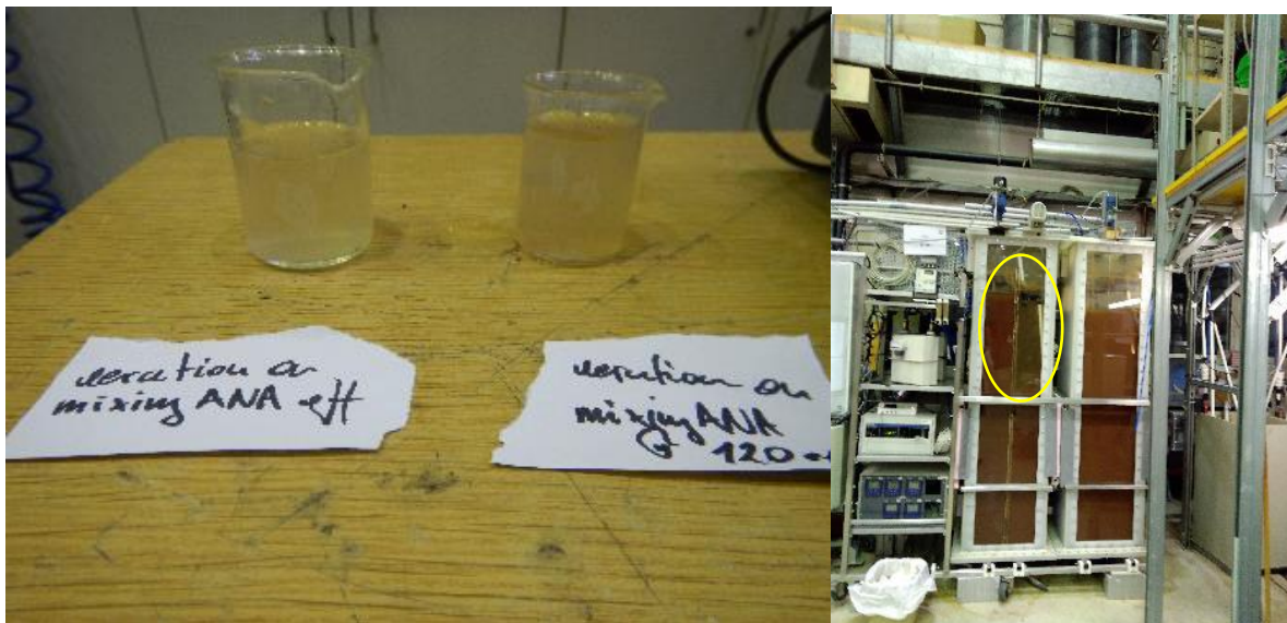
Figure 31: (Left) Effluent grab samples indicating good sludge retention during continuous operation; (right) sludge retention visible to the eye during continuous operation.
