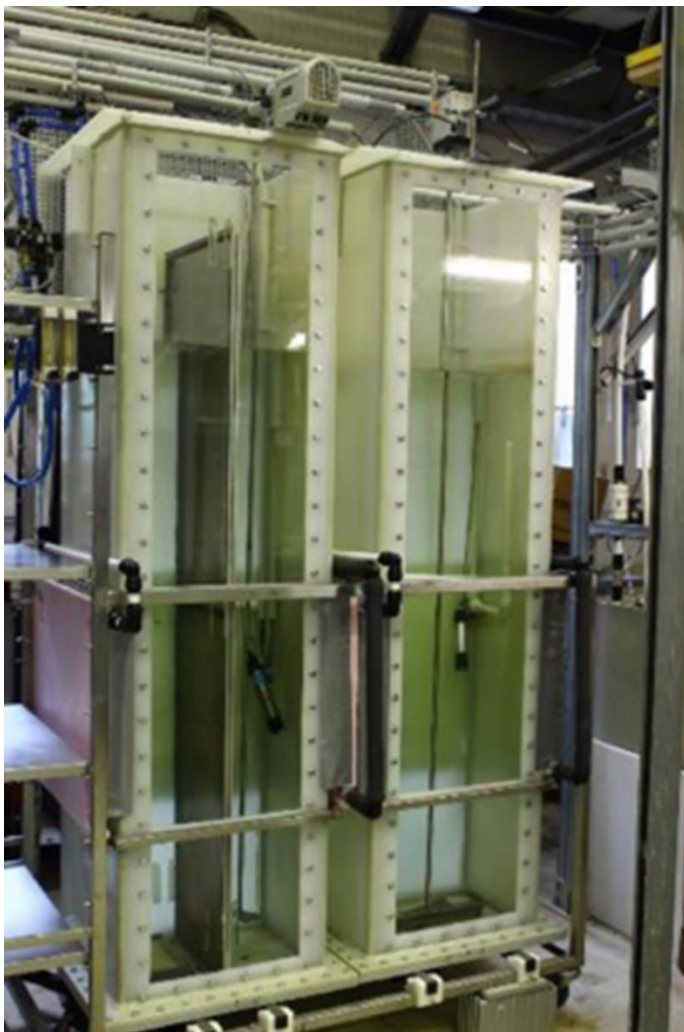
Figure 8: Pilot plant before start-up consisting of a single chamber (right) and a two-compartment mesh system (left) (Weissenbacher et al. 2017).
