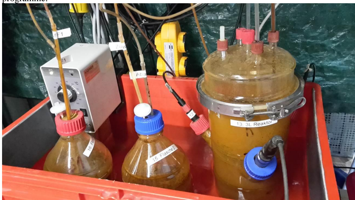
Figure 5: 3 L single chamber system (right) and 1.5 L batch test bottles (left); the red colour is due to increased iron concentrations.
