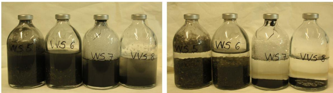
Figure 12: Anaerobe pre-test with saponin and nZVI to observe foaming w/o quartz sand; left side: directly after taking samples from shaker, right side: samples after 24 hours of resting; VVS 5 and VVS 7 with 0.1 \text{ g L}^{-1} of saponin ( >\text{CMC} ), VVS 6 and VVS 8 with 0.005 \text{ g L}^{-1} ( <\text{CMC} )
