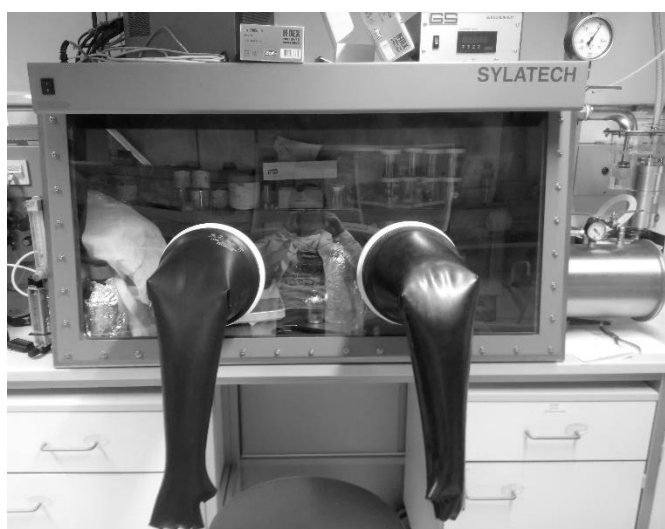
Figure 9: Glovebox used for preparing samples with port on the right side
