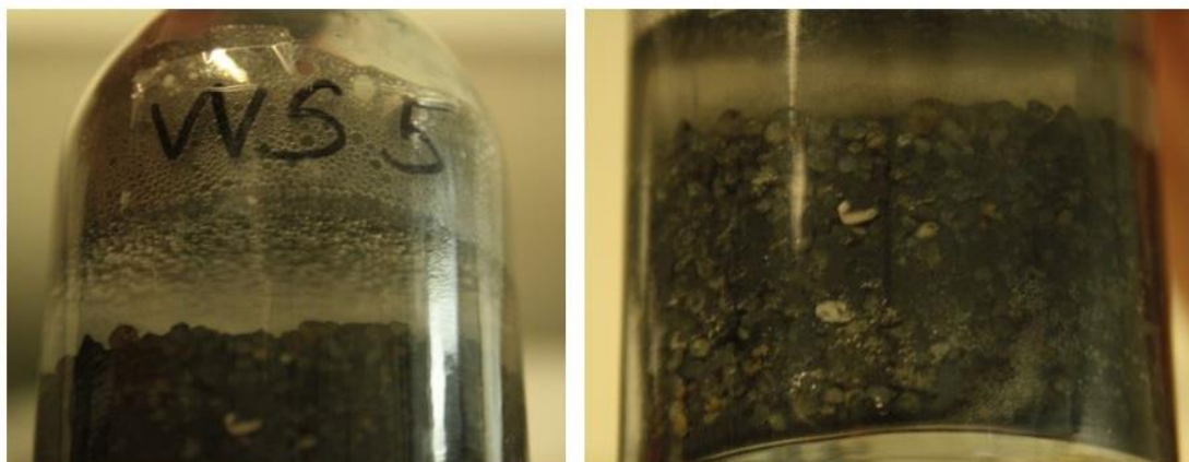
Figure 13: VVS 5 (high saponin concentration + quartz sand) after 26 hours (24 hours of shaking and 2 hours of resting), accumulated gas bubbles at bottom of foam (left side) and in pores of quartz sand (right side)
