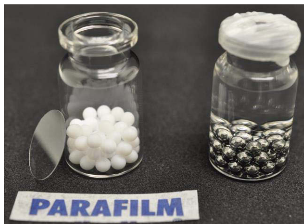
Figure 11: Worst-case small-scale for abrasion of adsorbed proteins consisting of a glass vial, spheres of a specific size and material and a cover glass that is closing the system and fixed by parafilm ®. Figure taken from publication II.
