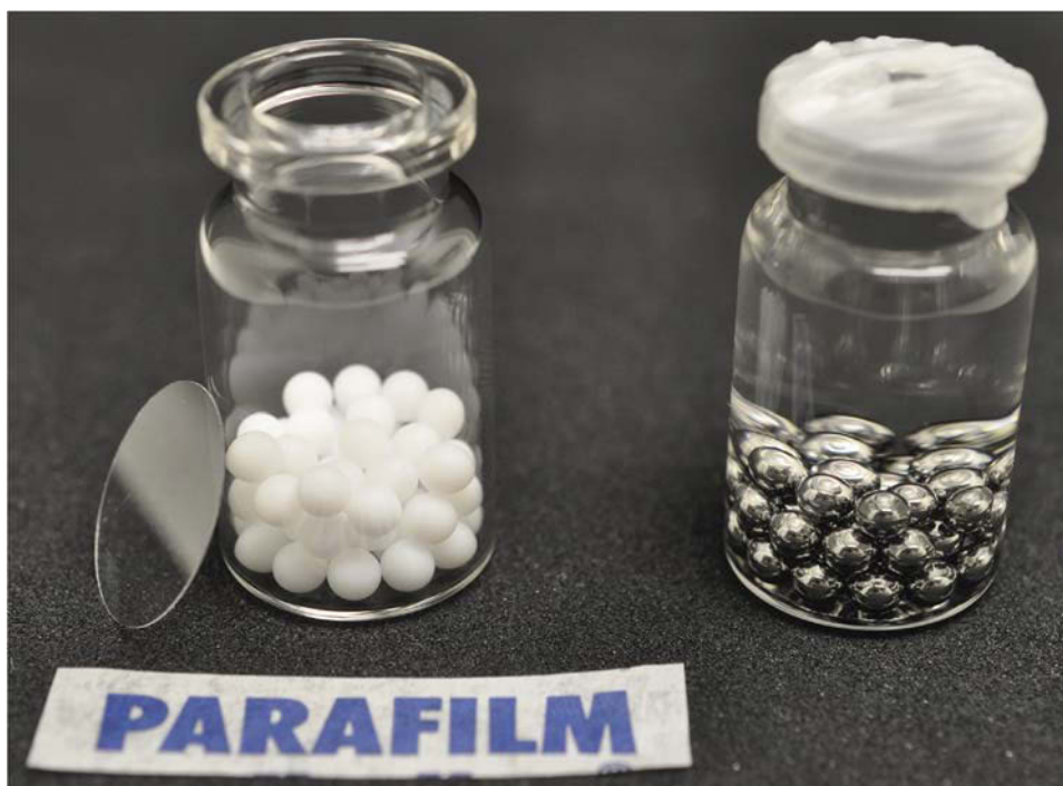
Fig. 3. Test system consisting of spheres inside a glass vial that is closed by a cover glass. The cover glass is fixed by wrapping parafilm around.
