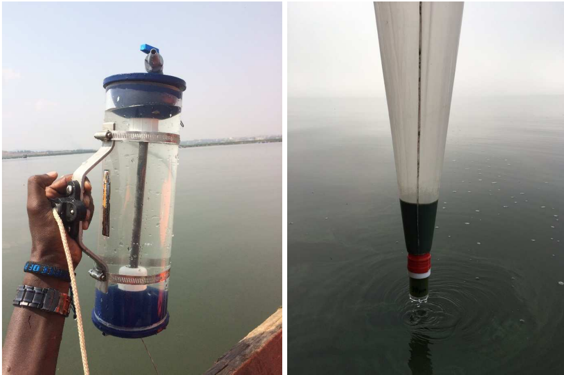
Figure 6: An integrated water sample in a 2-litre Van Dorn sampler from a known depth (Left) and concentrated water sample in a 30 µm plankton net (Right).
