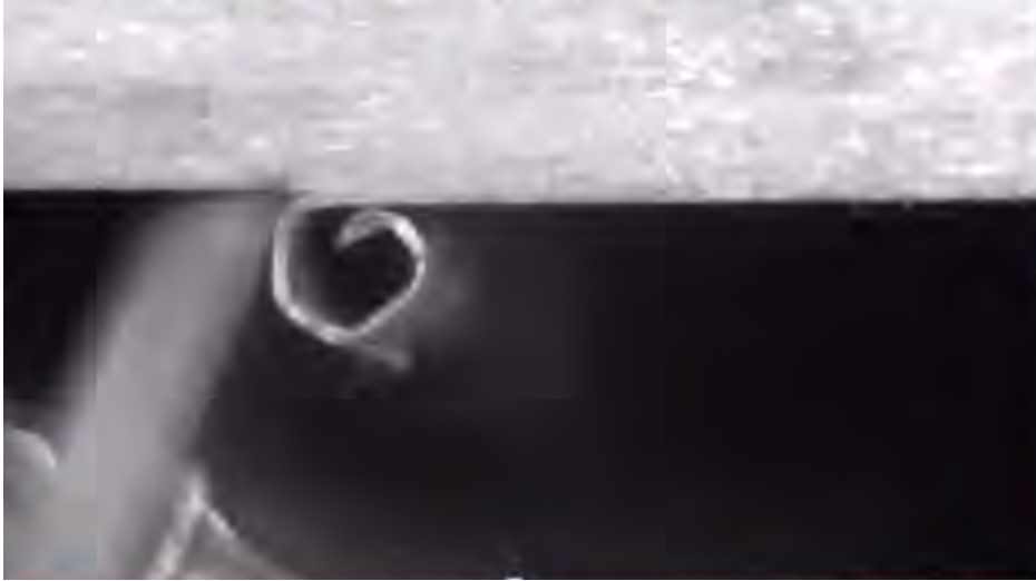
Figure 7: Segmented chip, produced by cutting with the angle between wood grain and cutting direction of 0^\circ , which was described by Kivimaa (1950) as cutting direction B.
