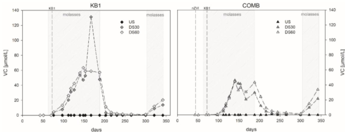
Fig. 6: Metabolite concentrations (TCE, cis-DCE and VC) at the sampling points upstream (US) and downstream (DS30 = 30 cm, DS60 = 60cm) of the treatment zone. The vertical dashed lines indicate injection times of nZVI and KB1. Hatched areas indicate the periods of molasses addition.
