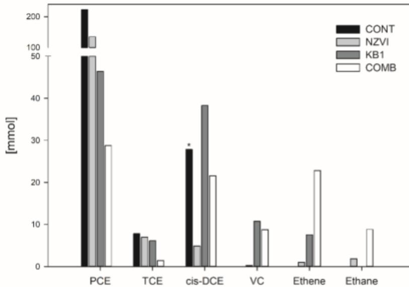
Fig. 2: Cumulative loads of PCE, metabolites and fully dechlorinated end products calculated from the volumes and concentrations of the efflux from each chamber. \* marks the metabolites formed only during molasses input in chamber CONT
