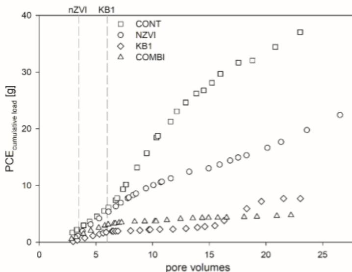
Fig. 3: Time course of PCE loads in the efflux of the chambers during the whole experiment. The vertical dashed lines indicate times of injection of nZVI and KB1. The hatched areas indicate the period of molasses addition into chambers KB1 und COMB. The dotted area indicates the period of molasses addition into chamber CONT.
