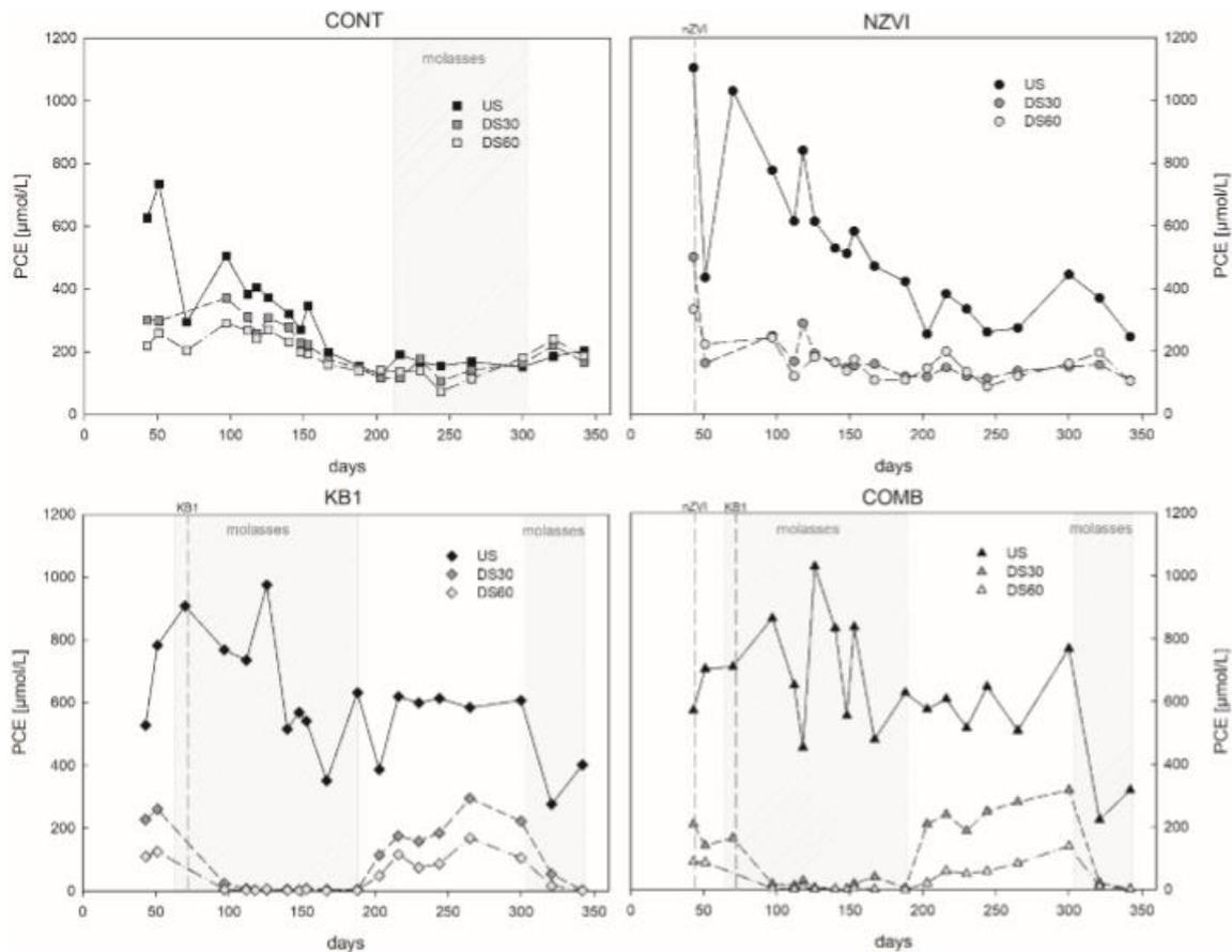
Fig. 4: PCE concentrations at the sampling points upstream (US) and downstream (DS30 = 30 cm, DS60 = 60cm) of the treatment zone. The vertical dashed lines indicate injection times of nZVI and KB1. Hatched areas indicate the periods of molasses addition.
