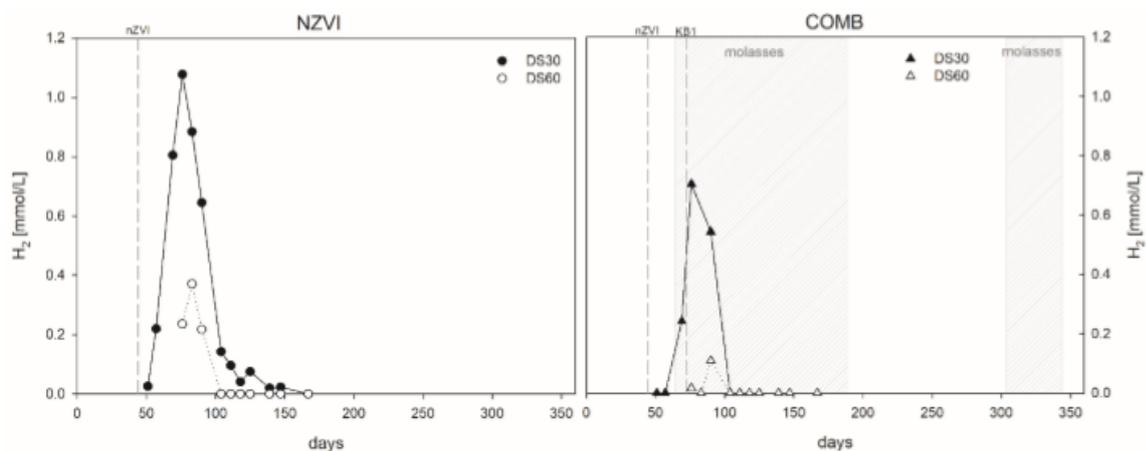
Fig. 7: H<sub>2</sub> concentrations at sampling points downstream (DS30 = 30 cm, DS60 = 60cm) of the treatment zone. The vertical dashed lines indicate injection times of nZVI and KB1. Hatched areas indicate the periods of molasses addition.
