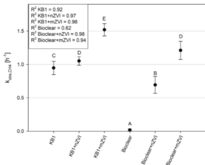
**Fig. 5.** Observed reaction constants ( $k_{\text{obs}}$ ) for the microbial formation of  $\text{CH}_4$  in all bacterial microcosms (KB1, KB1 + nZVI, KB1 + mZVI, Bioclear, Bioclear + nZVI and Bioclear + mZVI). Error bars represent standard deviations of three replicates. Different letters above the symbols indicate statistically significant differences between the respective values ( $\alpha = 0.05$  Duncan's post-hoc test).
