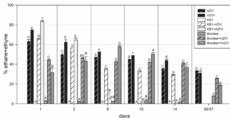
Figure S.1: Percentage of ethane and ethyne of the total amount of dechlorinated end products produced by all treatments (nZVI, mZVI, KB1, KB1+nZVI, KB1+mZVI, Bioclear, Bioclear+nZVI and Bioclear+mZVI). Error bars represent standard deviations of the three replicates. Different letters (A, B, C, ...) above the bars indicate statistically significant differences among treatments within one timepoint ( $\alpha = 0.05$ , Duncan post hoc test).
