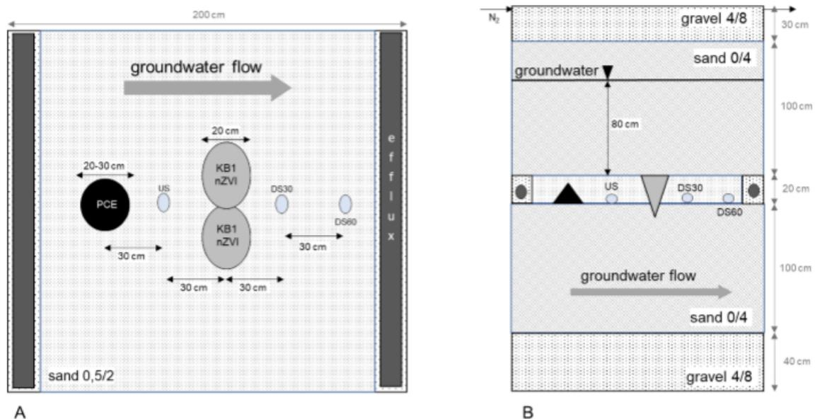
Fig. 1: (A) Horizontal and (B) Vertical layout of the simulated aquifer (depth 130-150 cm) in the lysimeter chambers and positioning of the sampling and injection tubes in the aquifer zone. Elements can vary according to the treatments of each chamber (PCE = PCE phase; treatment zone: Injection of nZVI and KB1-culture; US, DS30 and DS60 = sampling ports upstream, 30 cm and 60 cm downstream of the treatment zone).
