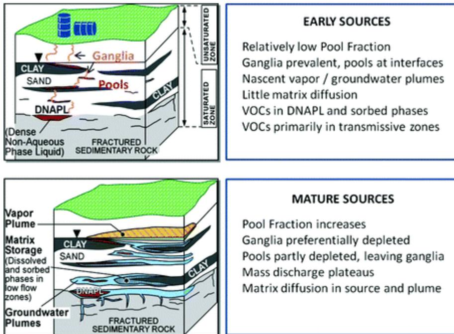
Figure 2: Behavior of DNAPL contamination in the underground (Stroo et al., 2012)
