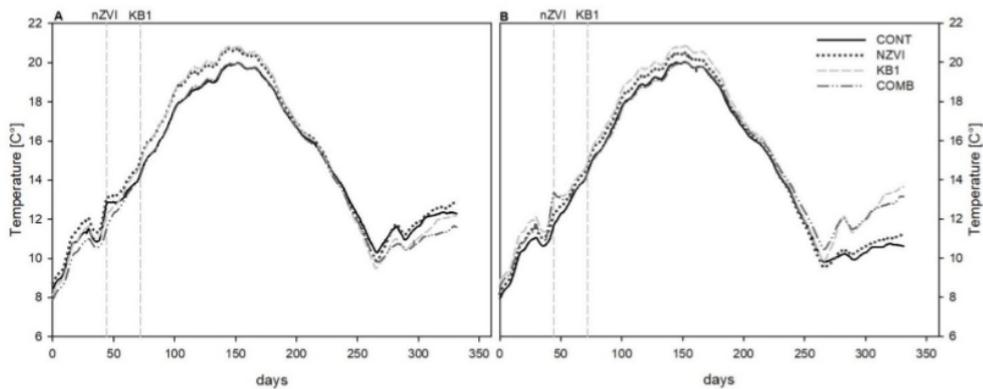
Fig. S.3: Temperature development before (A) and after (B) the treatment zones in chambers CONT, NZVI, KB1 and COMB (vertical dash lines indicating nZVI and KB1 injection)
