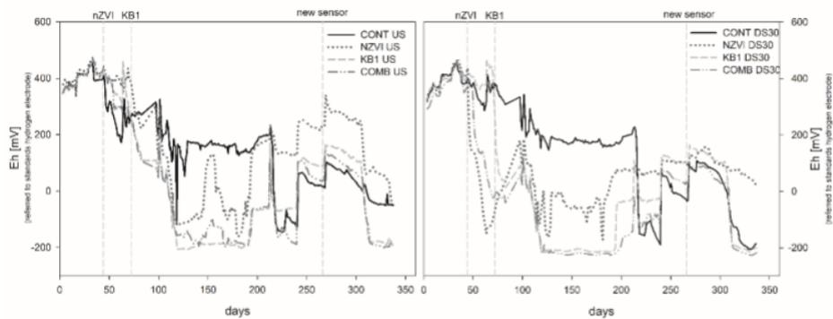
Fig. S.4: Eh (referred to standard hydrogen electrode) development at the sampling points US and DS30 of chambers CONT, NZVI, KB1 and COMB (vertical dash lines indicating nZVI and KB1 injection and installation of a new ORP sensor)
