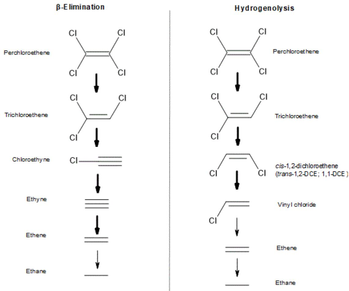
Figure 4: Main metabolites and products of  $\beta$ -elimination and hydrogenolysis during the abiotic PCE dechlorination by ZVI. Bolt arrows indicating fast reactions and thin arrows slower reactions.
