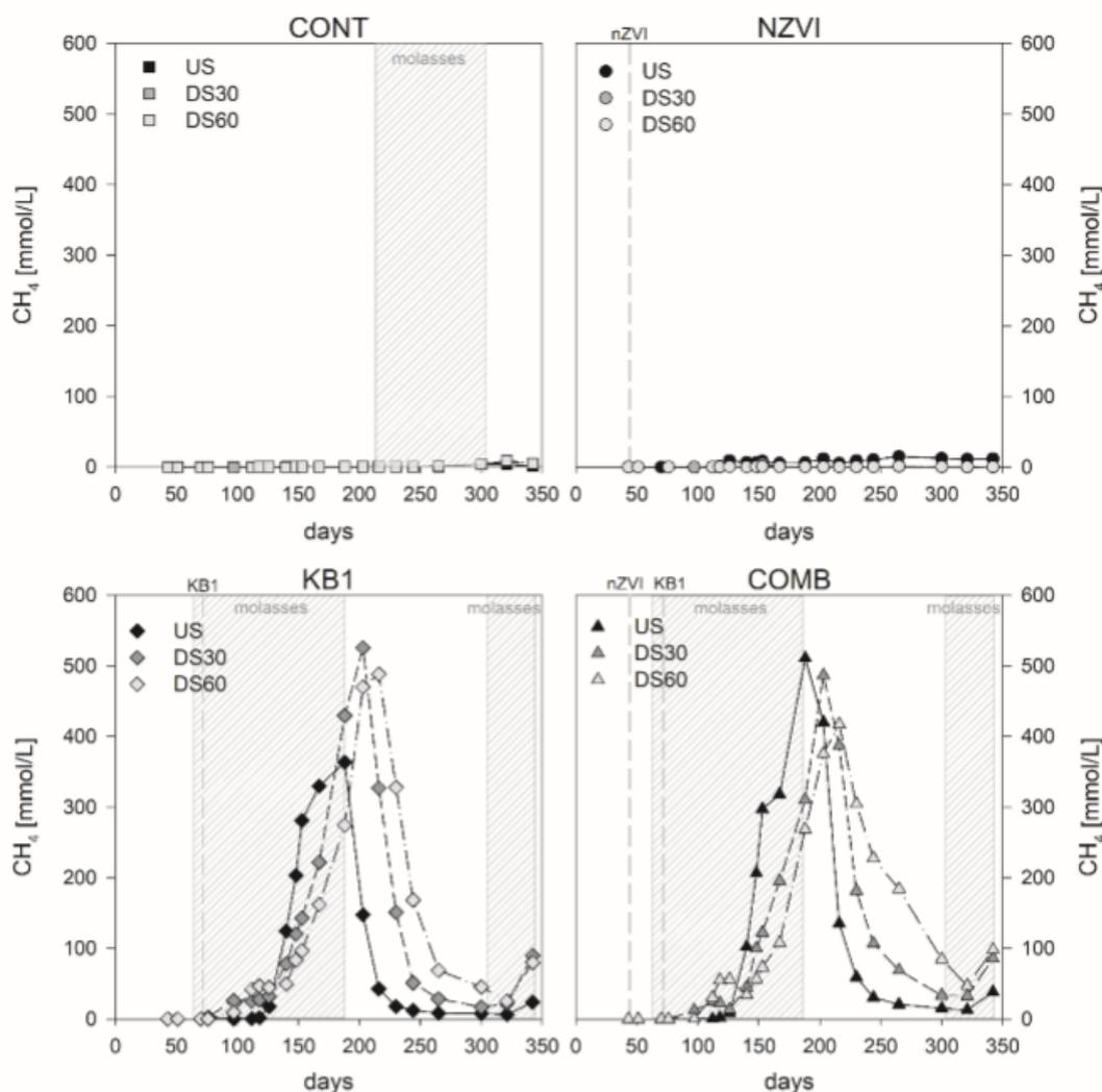
Fig. 8: CH<sub>4</sub> concentrations at sampling point upstream (US) and downstream (DS30 = 30 cm, DS60 = 60cm) of the treatment zone and in the effluent of each lysimeter chamber. The vertical dashed lines indicate injection times of nZVI and KB1. Hatched areas indicate the periods of molasses addition.
