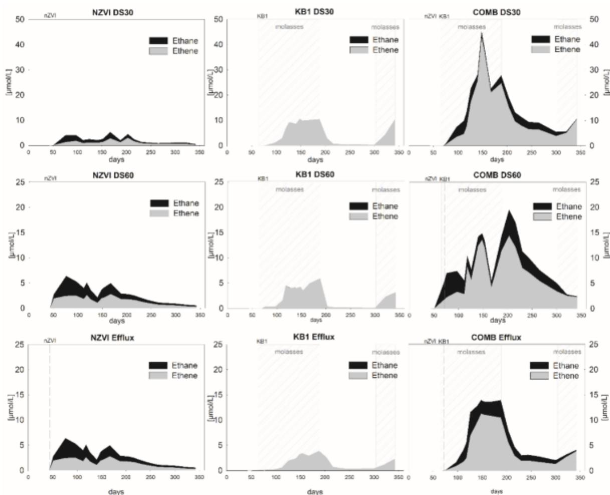
Fig. 5: Ethene and ethane concentrations at the sampling point DS30, DS60 and efflux of chambers NZVI, KB1 and COMB. The vertical dashed lines indicate injection times of nZVI and KB1. Hatched areas indicate the periods of molasses addition. The dotted lines shown in the three graphs for COMB indicate the sum of ethene+ethane concentrations measured in the chambers NZVI and KB1.
