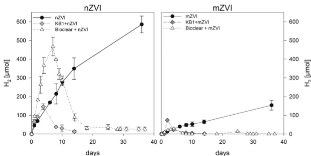
Fig. 3.  $\text{H}_2$  development in the treatments containing ZVI particles (nZVI, KB1 + nZVI, Bioclear + nZVI, mZVI, KB1 + mZVI, Bioclear + mZVI). Error bars represent standard deviations of three replicates.
