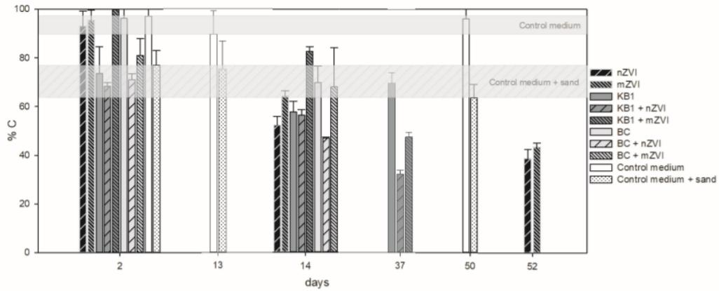
Figure S.2: Carbon balances of all treatments and the two control experiments at different time points (day 2, 13, 14, 37 and 50). The plain grey area and the hatched grey area show the lowest and the highest mean carbon recoveries of control 1 and control 2 respectively over the course of the experiment. Error bars represent standard deviations of the three replicates.
