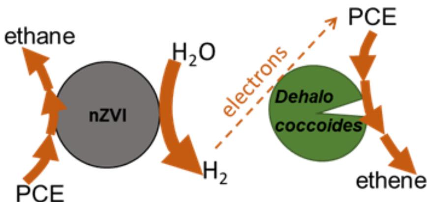
Figure 6: Schematic overview of the potential usage of ZVI produce  $H_2$  by dehalorespiring *Dehalococcoides* spp.
