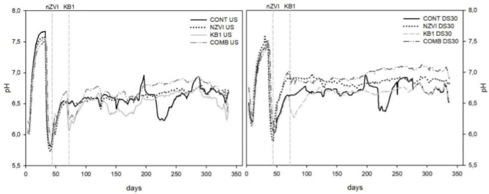
Fig. S.2: pH values at sampling points US and DS30 of chambers CONT, NZVI, KB1 and COMB (vertical dash lines indicating nZVI and KB1 injection)
