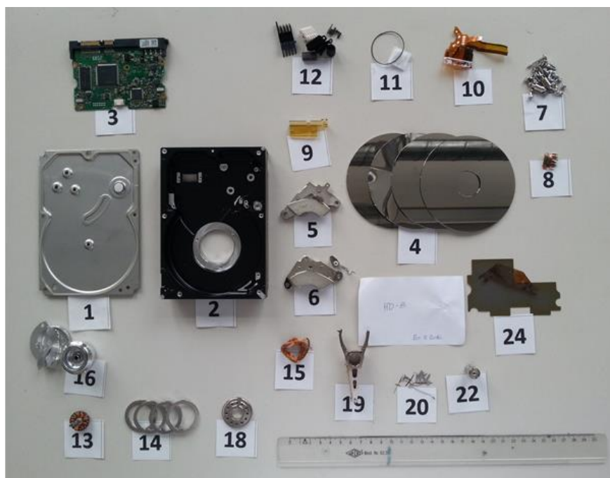
Figure 12: Example of disassembled HDD with labelled parts
