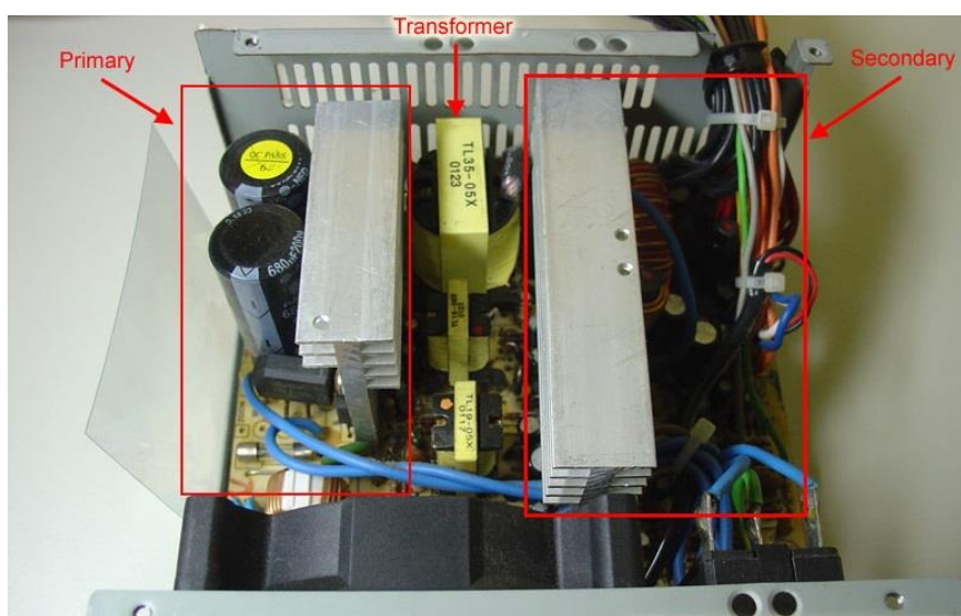
Figure 9: Structure of PSU from PC (Torres, 2006)
