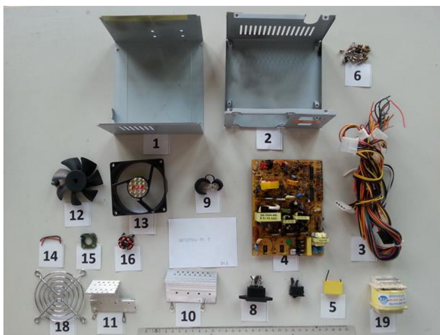
Figure 14: Example of disassembled PSU (PC) with labelled parts
