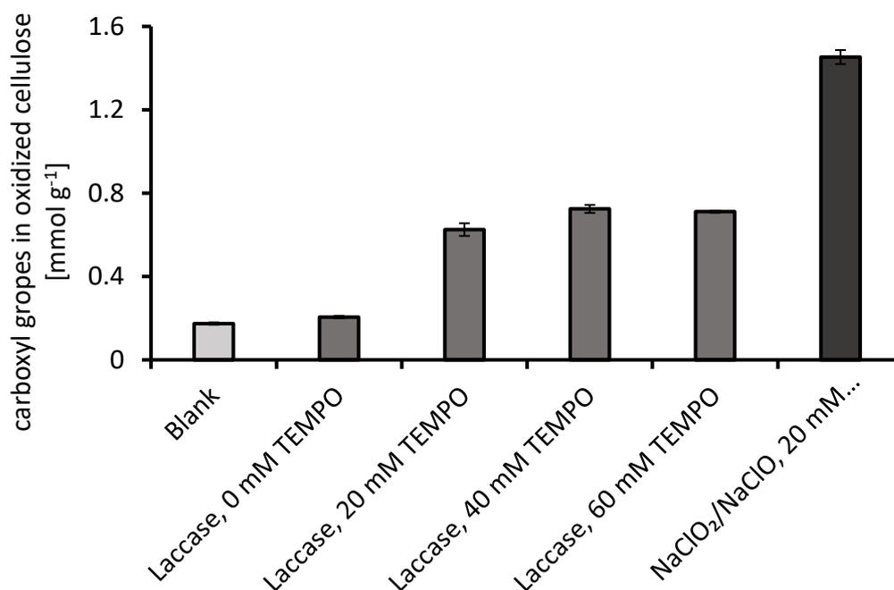
Figure 4. Influence of the TEMPO concentration on enzymatic oxidation of cellulose fibers in comparison to chemical oxidation. Blank is without TEMPO and without oxidation system (bright grey), enzymatic oxidation with laccase and different TEMPO concentration from 0 – 60 mM (middle grey) and chemical oxidation with NaClO<sub>2</sub>/NaClO and 20 mM TEMPO (dark grey). All experiments were performed in triplicates.
