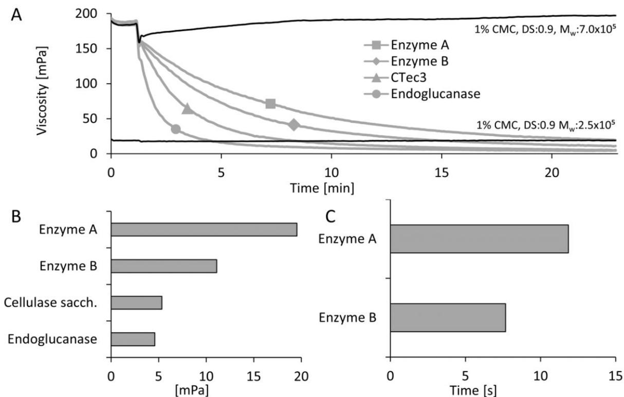
Figure 4. Viscosity profile of enzymes on a 1% CMC solution (DS 0.9,  $M_w 7.0 \times 10^5$ ) recorded for 24 min (A). end viscosity in mPa of Enzyme A, Enzyme B, Endoglucanase and CTec3 (B). Time one ml undiluted enzyme needed to degrade a 1% CMC with a DS0.9 &  $M_w 7.0 \times 10^5$  down to a viscosity comparable to a 1% CMC with a DS0.9 &  $M_w 2.5 \times 10^5$  (C).
