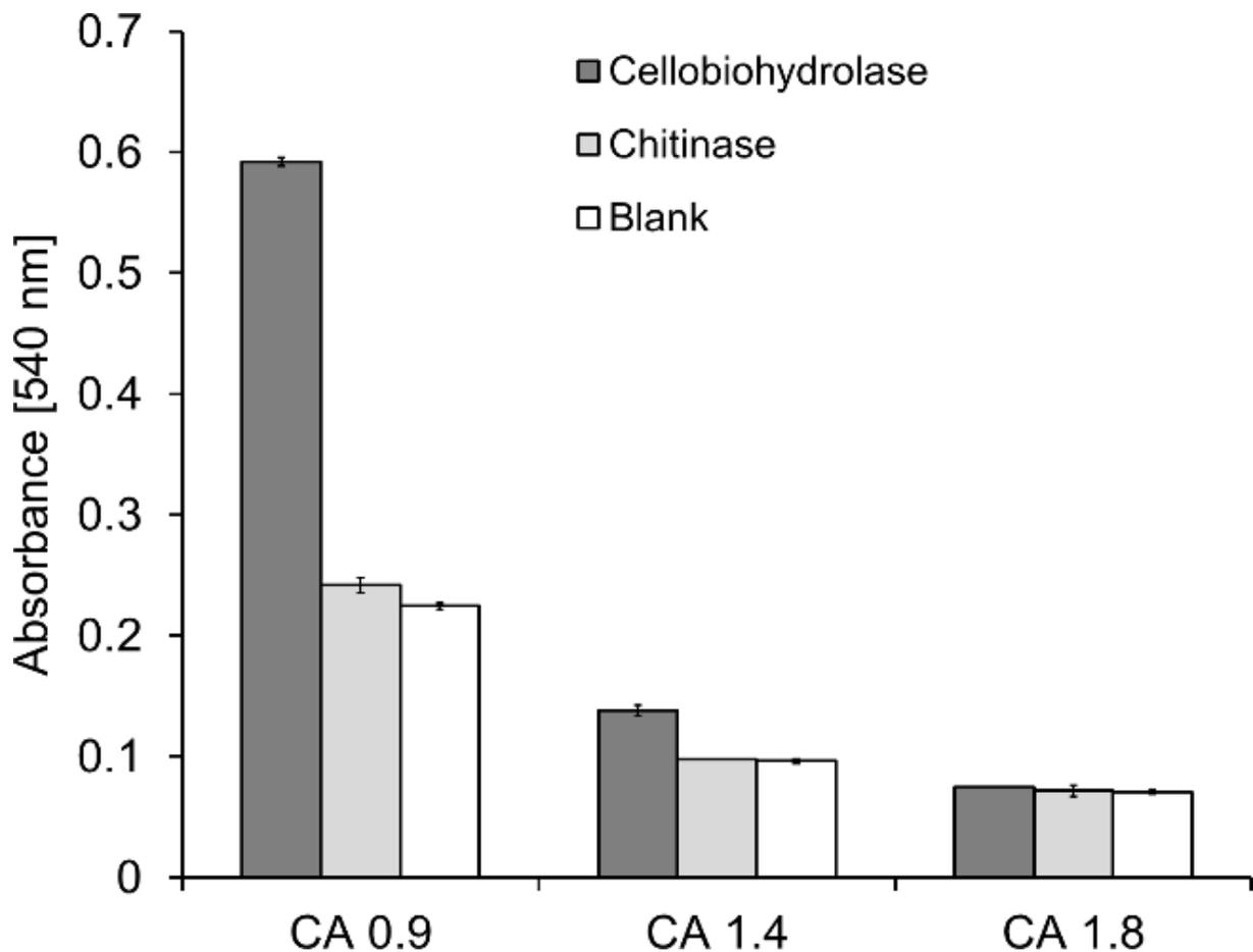
Figure 7. Backbone cleavage of cellulose acetates with chitinase and cellobiohydrolase I after 145 h.
