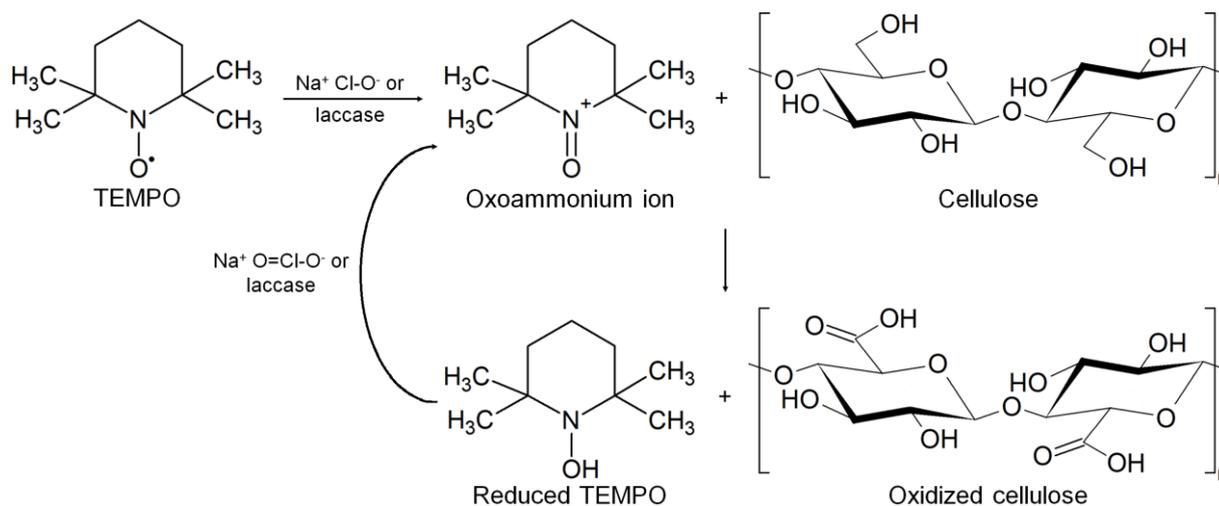
Figure 1. Oxidation of cellulose at the C6 position. Formation of the oxoammonium ion from TEMPO with  $\text{NaClO}$  (chemical) or laccase (enzymatic). The oxoammonium ion oxidizes cellulose and is then recycled by  $\text{NaClO}_2$  (chemical) or laccase (enzymatically).
