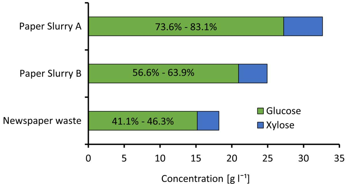
Figure 4. Glucose and xylose concentration of larger scale hydrolysis (1.5 l stirred reactor) of newspaper waste, Paper Slurry A and Paper Slurry B (75 g l<sup>-1</sup>) with CellicCtec3 (5%) at 50 °C and pH5. Numbers in the green bars indicate glucose recovery based on the cellulose content given in Figure 1.
