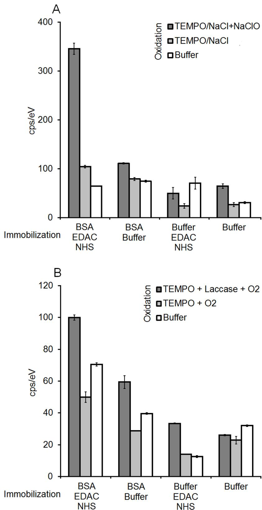
Figure 9. Variations in nitrogen concentration after EDAC/NHS covalent coupling of BSA to chemically oxidized (A) and enzymatically oxidized cellulose (B). Nitrogen concentration on the cellulose fibers was monitored using SEM (Hitachi 3030, Japan) and the software Quantax 70 (Bruker, United States).
