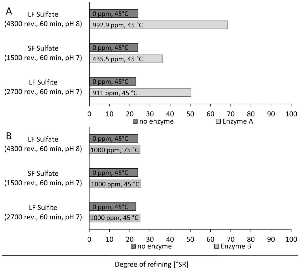
Figure 7. Comparison of refining degree for LF Sulfate, SF Sulfate and LF Sulfite pulp at different conditions. Strong effects are visible for Enzyme A (A), weak effects are visible for Enzyme B (B). Strongest effects are visible for LF Sulfate pulp for Enzyme A.
