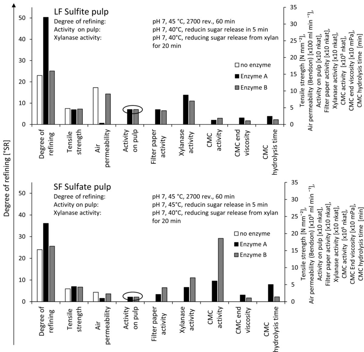
Figure 8. Comparison of pulp and paper parameters (degree of refining, tensile strength, air permeability) with enzyme characteristics (activity on pulp, filter paper activity, xylanase activity, CMC activity, CMC hydrolysis time). The enzymes were dosed according to their activity on pulps (elliptic line, Activity on pulp). LF Sulfite pulp: 1000 ppm Enzyme B, 911 ppm Enzyme A. SF Sulfate pulp: 1000 ppm Enzyme B, 435.4 ppm Enzyme A.
