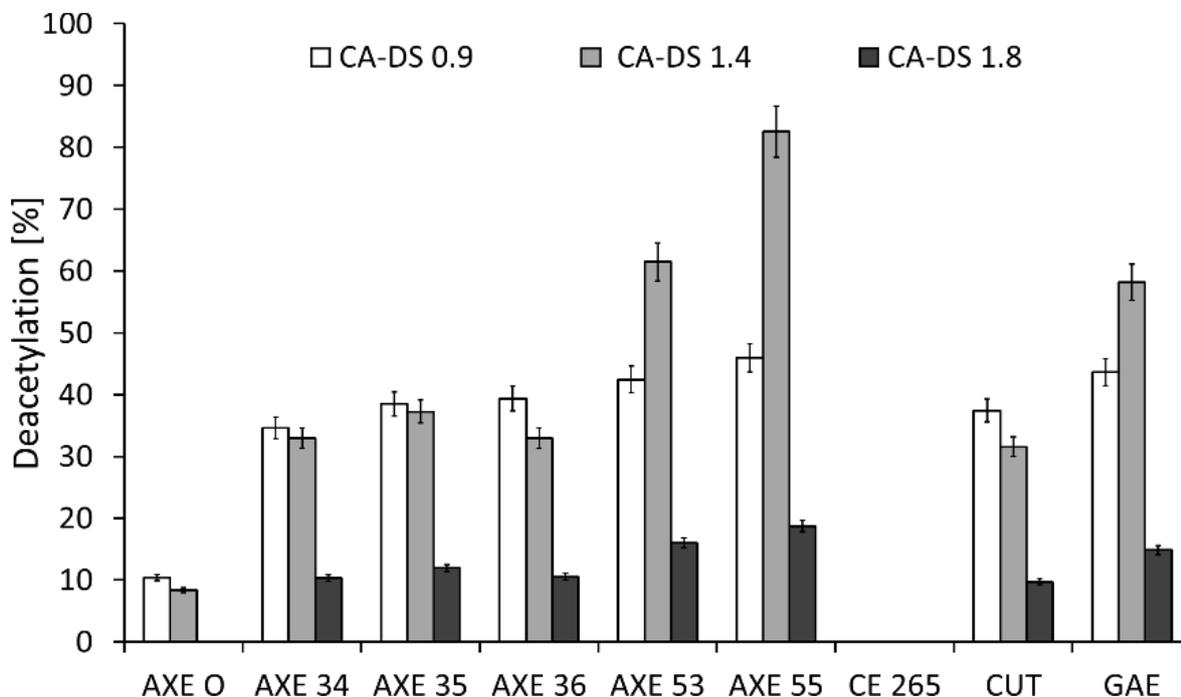
Figure 4. Deacetylation of different cellulose acetates by esterases. Cellulose acetate with 0.9 acetyl groups per monomer (CA-DS 0.9), cellulose acetate with 1.4 acetyl groups per monomer (CA-DS 1.4) and cellulose acetate with 1.8 acetyl groups per monomer (CA-DS 1.8). Axetyl Xylan Esterase (AXE), Carbohydrate Esterase (CE), Cutinase (CUT), Glucomannan Acetyl Esterase (GAE), Pectin Acetyl Esterase (PAE).
