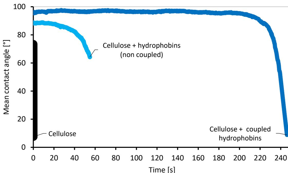
Figure 10. Hydrophobicity of fibers. Contact angle measurements of cellulose surfaces formed from fibers after chemical oxidation and hydrophobins coupling.
