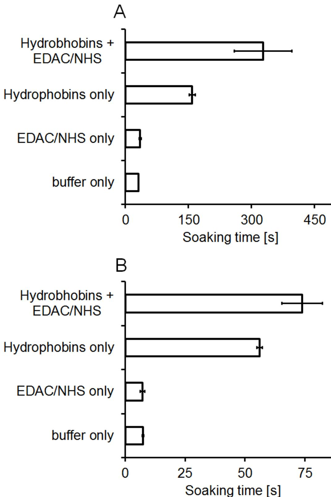
Figure 7. Hydrophobicity determination for cellulose surfaces covalently functionalized with hydrophobins subsequently to prior chemical oxidation of cellulose. Soaking time determination using contact angle measurements for various paper surfaces. Paper containing 6-7% lignin (A) and paper composed of 100% cellulose (B).
