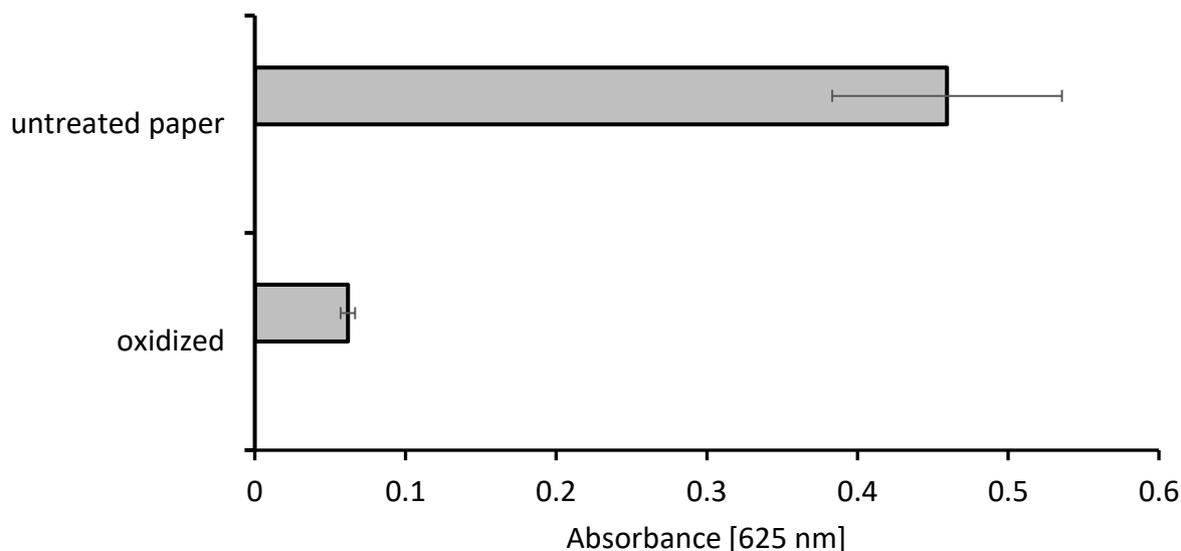
*Figure 5. Qualitative analysis of carboxylic groups introduced into paper sheets via TEMPO/sodium hypochlorite. Unbound toluidine blue after staining was photometrically determined in the washing water after two rinsing steps.*
