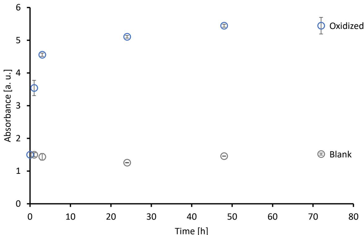
Figure 6. Chemical oxidation of a Kraft White cellulose surface with sodium hypochlorite and TEMPO for 72 h as quantified by FTIR at a wavelength of  $1605\text{ cm}^{-1}$  (normalization from  $2850\text{-}2950\text{ cm}^{-1}$ ). All experiments were performed in triplicates.
