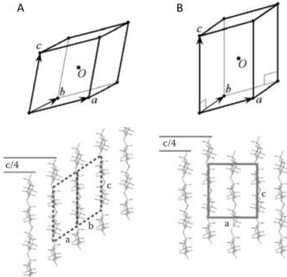
Figure 3. Three-dimensional crystal structure of a triclinic (A) and monoclinic (B) crystal system with the corresponding cellulose type cellulose Ia (A) and Ib (B). The vectors are indicated by  $a$ ,  $b$  and  $c$ . The center point is  $O$ . The crystal structure for the repeating unit (cellobiose) is marked as grey box for cellulose Ib and as dotted box for cellulose Ia. Shift of neighboring chains is labeled as  $c/4$ . Figure adapted from [20] and [18].
