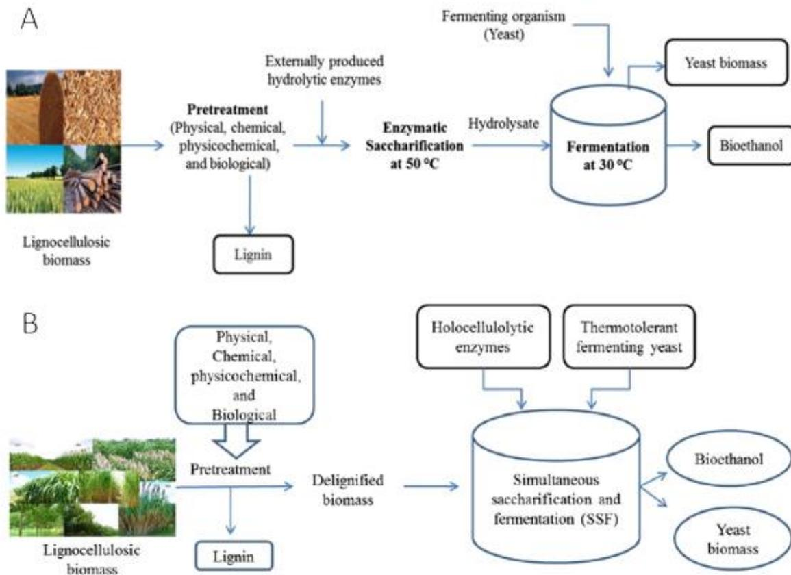
Figure 18. Process flow of separate hydrolysis and fermentation (SHF) (A) and simultaneous saccharification and fermentation (SSF)(B) [107].
