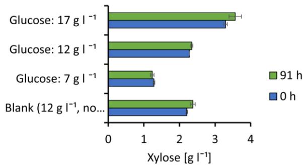
Figure S1. Xylose concentration in the beginning and after 91 h of heterotrophic algae cultivation on Paper Slurry A and Paper Slurry B. No significant consumption was visible for both slurries at all measure glucose levels. Error bars indicate standard deviation of biological duplicates.
