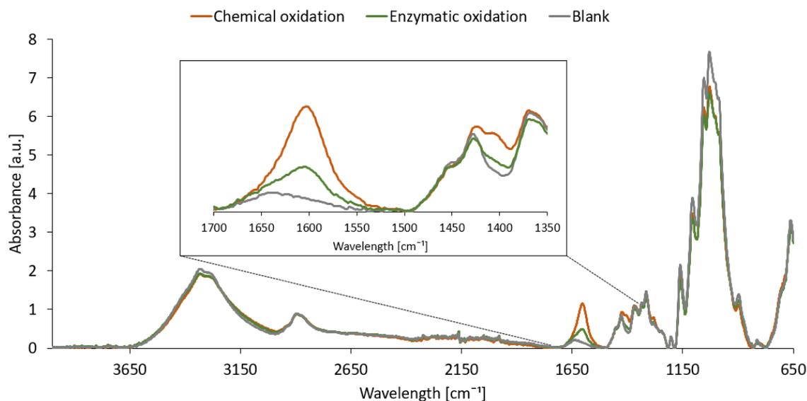
Figure 3. FT-IR monitoring of the chemical (A) and enzymatic (B) oxidation of cellulose fibers using TEMPO as mediator. Spectra were baseline corrected and normalized in the  $2850\text{-}2950\text{ cm}^{-1}$  area and the determination of the carboxylic content was performed according to the absorbance at a wavelength of  $1610\text{ cm}^{-1}$ . Chemical oxidation was conducted for 24 h and enzymatic oxidation for 48 h.
