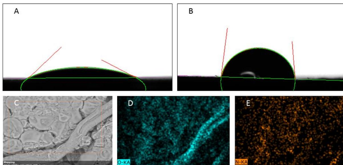
*Figure 8. Coupling of hydrophobins to chemical oxidized Whatman No.1 filter paper. Contact angle measurement (A-B) and SEM imaging (C-E) for paper sheets oxidized and EDAC/NHS coupled hydrophobins, Contact angle for non-oxidized material treated with hydrophobins (A), contact angle for oxidized and coupled surface (B), SEM image of a paper fiber with coupled hydrophobins (C), distribution of oxygen for the fiber visible before (D), nitrogen distribution for the same fiber (E).*
