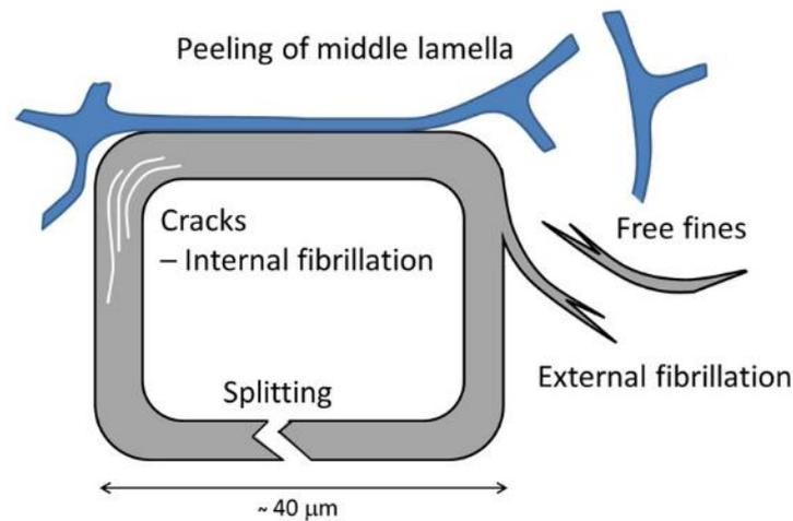
Figure 17. Internal and external fibrillation of cellulose caused by mechanical force. Internal fibrillation [94].
