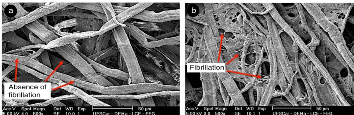
Figure 8. Scanning electron microscopy (SEM) of unrefined (a) and refined (b) bleached eucalyptus fibers [45].
