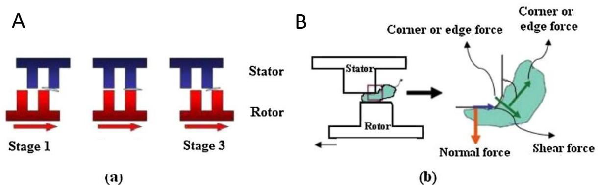
Figure 9. Refining mechanism for a single fiber between the bars of a rotor (red) and a stator (blue) in a refiner (A). Type and direction of forces present within a single fiber during refining (B) [41].
