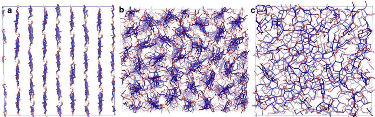
Figure 4. Simulated crystalline structure of cellulose in a temperature range from 250 (a) to 650 K (b), over a total recording time of 9 ns. Crystalline  $\beta$  cellulose (a), paracrystalline cellulose (b) and amorphous cellulose (c). The simulation box is given as square around the cellulose [24].
