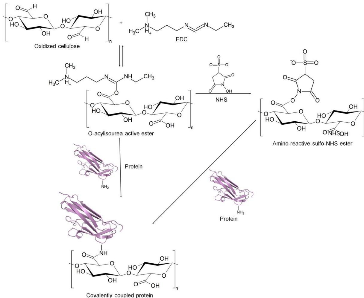
Figure 2. EDC/NHS coupling of proteins to oxidized cellulose. EDC couples to COOH groups of oxidized cellulose resulting in an active ester. In the presence of NH<sub>2</sub>-groups a covalent amide bond with a protein, or hydrolysis back to oxidized cellulose is possible. With NHS the active ester can form an Amin-reactive sulfo-NHS ester, which results in covalent bonds to NH<sub>2</sub>-groups of proteins.
