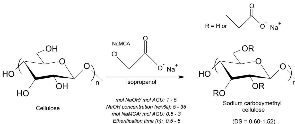
Figure 12. Production of carboxymethyl cellulose from cellulose. An alkalization with NaOH in isopropanol is followed by an etherification with monochloroacetate [59].
