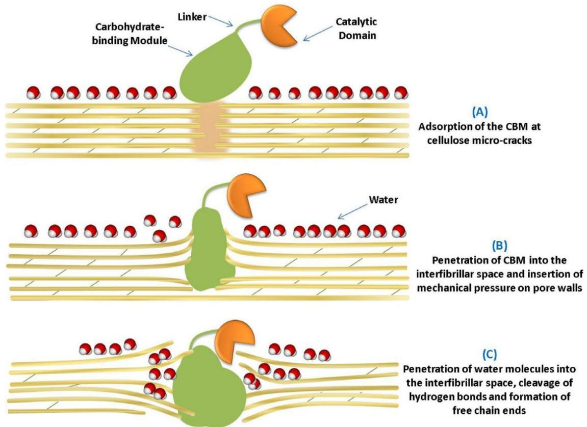
Figure 14. Schematic representation of an enzyme active on cellulose, carrying a cellulose binding module (CBM) linked to the catalytic domain. Further, the three steps of amorphogenesis of cellulose which are adsorption (A), penetration of CBM (B) and cleavage of hydrogen bonds by penetrating water (C) [73].
