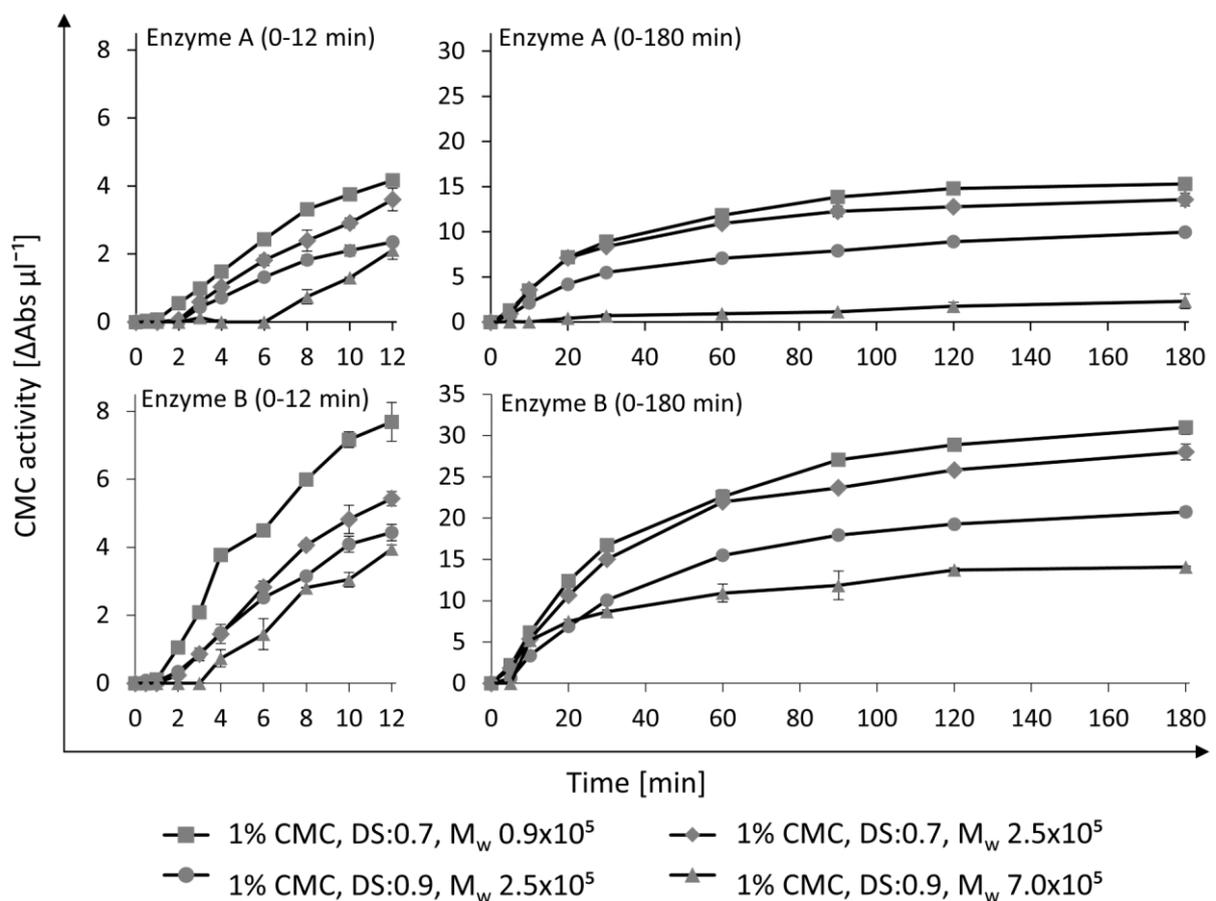
Figure 5. Enzymatic hydrolysis of CMC with different degree of substitution (DS) and polymerization ( $M_w$ ), for two different timeframes by refining enzyme preparations A and B. Longer chain length and higher degree of substitution caused less hydrolysis. Enzyme B was slightly more active than Enzyme A.
