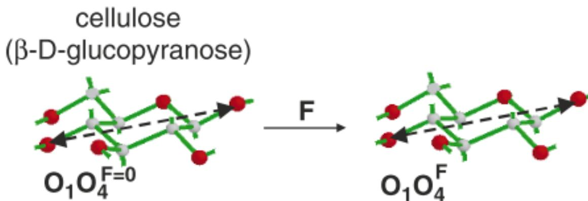
Figure 2. Typical chair formation of a glycopyranose ring in cellulose. Oxygen atoms are marked in red, carbon atoms are grey and bonds are green. Absence of a conformation changes when a force ( $F=0 \rightarrow F$ ) is indicated on the right. The distance of  $O_1O_4$  does not change, causing high rigidity of the cellulose chain [14].
