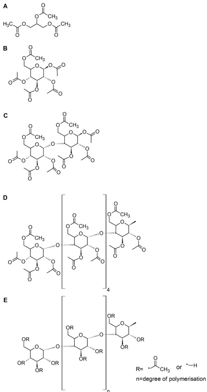
Figure 1. Substrates for enzymatic CA degradation. Triacetin (A), Glucose Pentaacetate (B), Cellobiose octaacetate (C), Hellohexose eicosacetate (D) and CA (E). For CA: R refers for the degree of substitution and  $n+2$  is the degree of polymerization.
