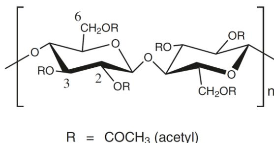
Figure 11. Structure of cellulose acetate (CA). Acetyl groups can be found on position C2, C3 and C6 of the backbone [51].
