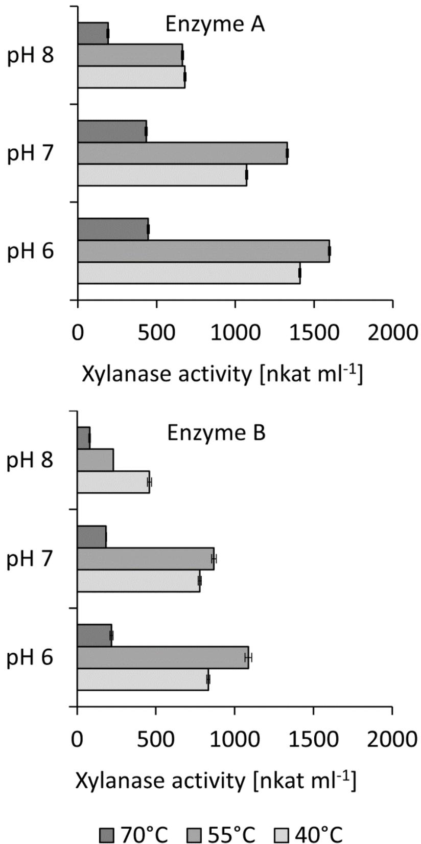
Figure 3. Xylanase activity for Enzyme A and B at a pH range from 6-8 for three different temperatures (40, 55 and 70 °C). Highest xylanase activity was visible for pH 6 and 55°C. Error bars indicate standard deviation of the performed triplicate.
