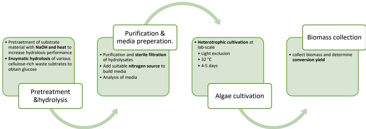
Figure 2. Scheme of the enzymatic substrate hydrolysis and digestate processing for heterotrophic algae cultivation.
