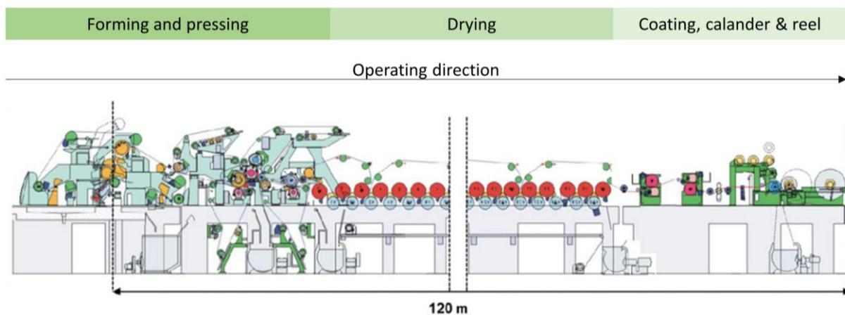
Figure 10. Paper machine, producing an endless paper sheet with up to  $130 \text{ km h}^{-1}$ . A pulp slurry is applied on the left and transported across the machine. Water is removed, in the beginning by vacuum and pressing forces (forming and pressing) and later by thermal drying (drying). With several techniques, other materials can be applied to the paper to change the sheet properties and surface characteristics. Finally the endless paper band is rolled up on a spindle on the right [47].
