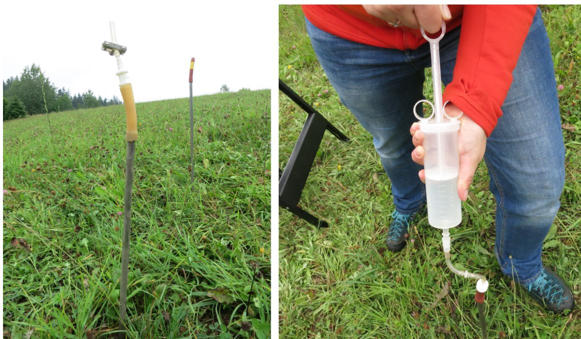
The first sample of soil air is discarded to avoid dilution with air already in the hollow part of the probe. Each sample is measured for at least four 10-minute-cycles, again discarding the first measurement result. This eliminates the effect of thoron on the radon measurement, as it will have decayed almost completely after the first 10 min measurement because of its short half-life.
