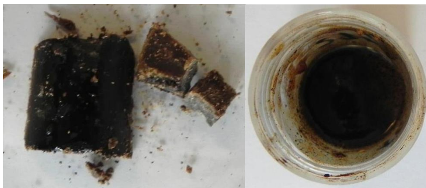
Figure 47 - Plastic mixture (B) pyrolyzed at 344 °C - solid/brittle fraction (left), waxy/liquid fraction (right)
