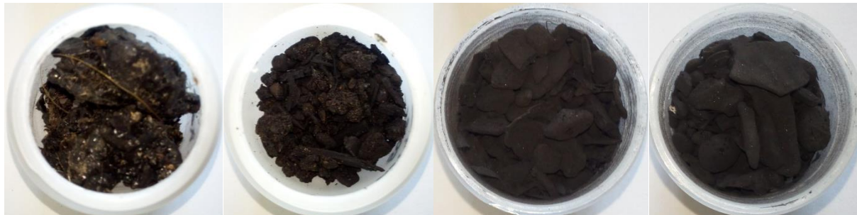
Figure 89 - Residues of the sea plastic pyrolyzed at 344 °C, 434 °C, 525 °C and 615 °C
