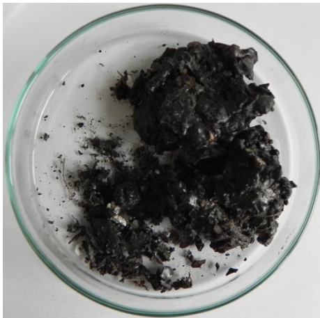
Figure 84 - Pyrolysis residue of sea plastic pyrolyzed at 344 °C
