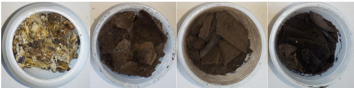
Figure 88 - Residues of the plastic mixture (A) pyrolyzed at 344 °C, 434 °C, 525 °C and 615 °C
