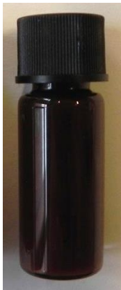
Figure 63 - Liquid/waxy product of plastic mixture (B) pyrolyzed at 615 °C
