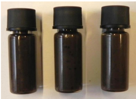
Figure 58 - Sea plastic pyrolyzed at 434°C (left), 525°C (middle) and 615°C (right)
