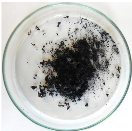
Figure 62 - Residue of plastic mixture (B) pyrolyzed at 615 °C and 60 minutes
