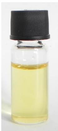
Figure 64 - Plastic mixture (B) pyrolyzed at 615 °C, distilled at 250 °C
