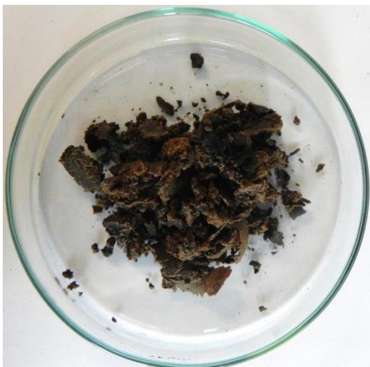
Figure 60 - Residue of the plastic mixture (B) pyrolyzed at 400 °C and 200 minutes
