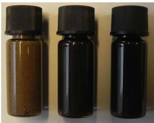
Figure 57 - Plastic mixture (A) pyrolyzed at 434 °C (left), 525°C (middle) and 615°C (right)
