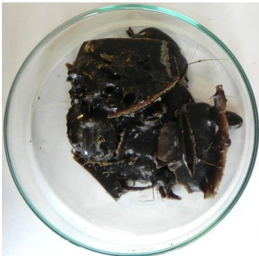
Figure 59 - Residue of the plastic mixture (B) pyrolyzed at 344 °C and 180 minutes
