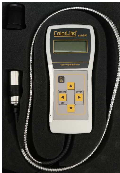
Figure 28: ColorLite sph850 Spectrophotometer
