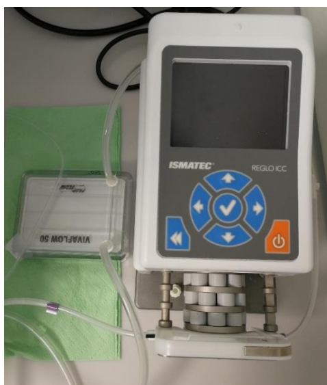
Figure 25: Vivaflow pump with 5 kDa cut-off membrane connected
