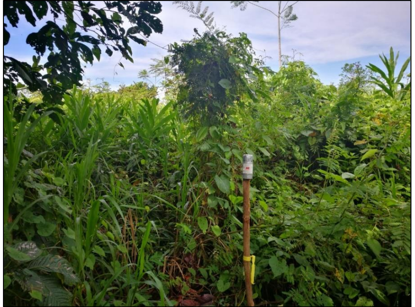
Fig. 10: Our reflective tool (toilet paper roll with reflective 3M tape mounted on a pole at breast height) used to create a reference point for tree position measurement (Own photo)
