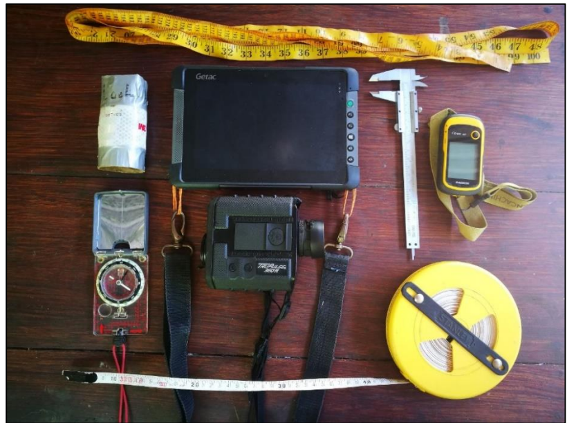
Fig. 11: Our field equipment used for height, diameter, crown, and position measurements (Own photo)
