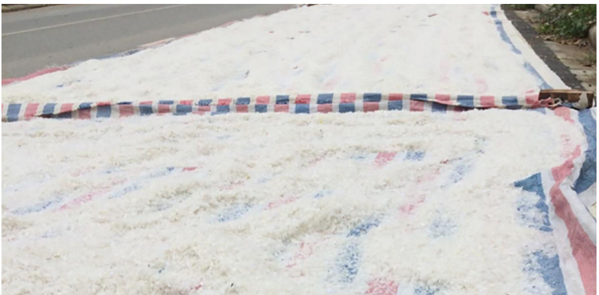
Figure 17: plastic flakes drying in the sun after washing (DesRoberts, 2017)
