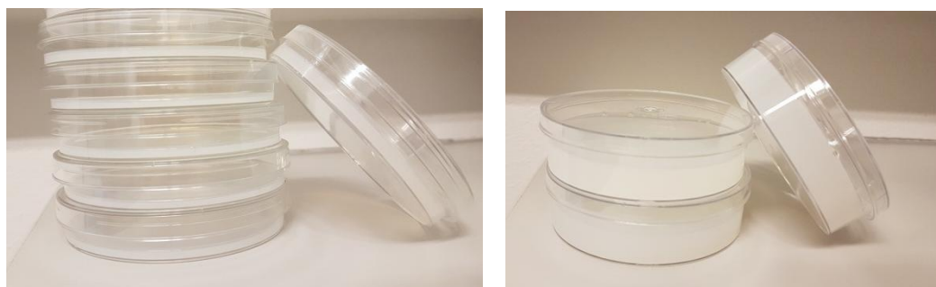
Figure 12: CAH-spiked silicone samples before cutting; left: thin layer for smooth cutting surface; right: thick layer for rough cutting surface
