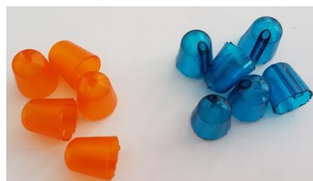
Figure 17: Dye-spiked and 3D-printed acrylic shells provided by Sonova
