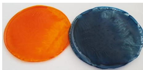
Figure 16: Dye-spiked TPU polymer samples provided by Sonova
