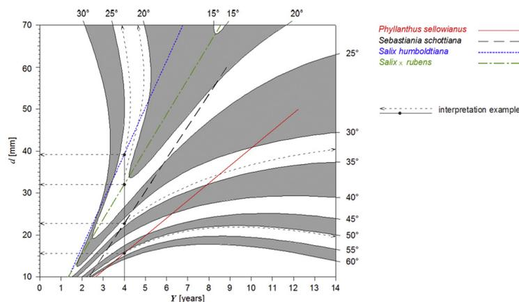
Fig. 6. Relationship with the diameter ( $d$ ) and angle of inflection at ultimate load ( $\alpha_u$ ), for different ages ( $Y$ ).
