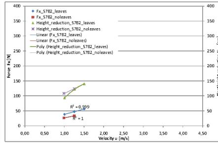
Fig. 15: Correlation between  $u$ ,  $F_x$  and  $H_{pr}$  for Salix 7 branch 2 in leafy and defoliated condition
