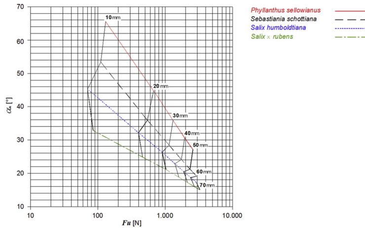
Fig. 5. Relationship between angle of inflection  $\alpha_u$  at rupture and  $\log F_u$  (ultimate load) dependent from the diameter for the four species.
