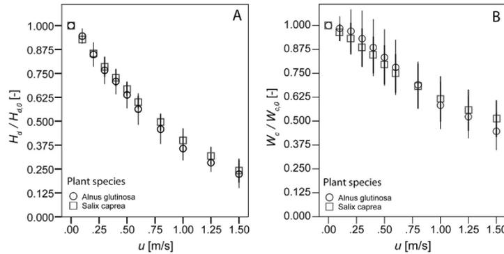
**Fig. 8.** Species-averaged deflected height  $H_d/H_{d,0}$  (A) and contracted width  $W_c/W_{c,0}$  (B) for *A. glutinosa* and *S. caprea* in foliated conditions. Measured velocities were 0.1–1.5 m/s. Error bars show  $\pm 1$  standard error.
