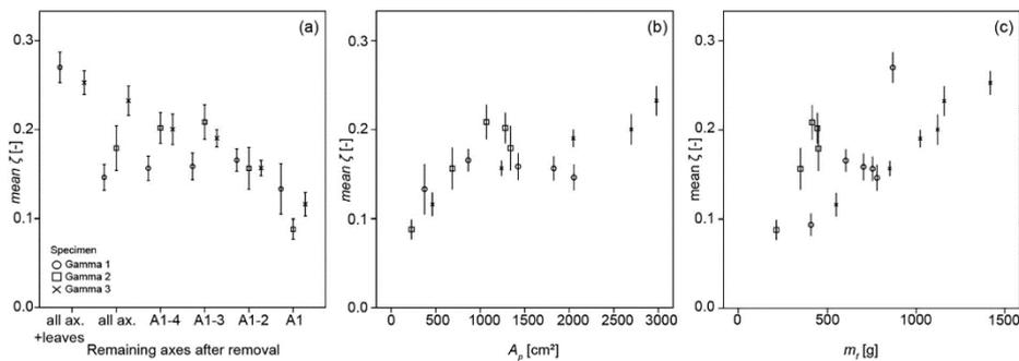
Fig. 7. Mean damping ratio ( $\zeta$ ) at different pruning steps (a). Interrelation between mean  $\zeta$  and the projected axes area ( $A_p$ ) (b) and between mean  $\zeta$  and fresh biomass ( $m_f$ ) of the specimens (c). Values in (b) and (c) represent damping ratios at the different pruning steps. Error bars show  $\pm 2$  standard error.
