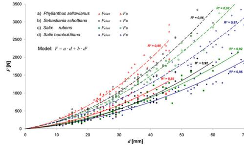
Fig. 2. Relationship between diameter ( $d$ ) and load ( $F$ ). Solid line: at the proportional limit,  $F_{elast}$ ; dashed line: at the ultimate load,  $F_u$ .
