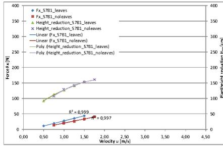
Fig. 14: Correlation between  $u$ ,  $F_x$  and  $H_{pr}$  for Salix 7 branch 1 in leafy and defoliated condition
