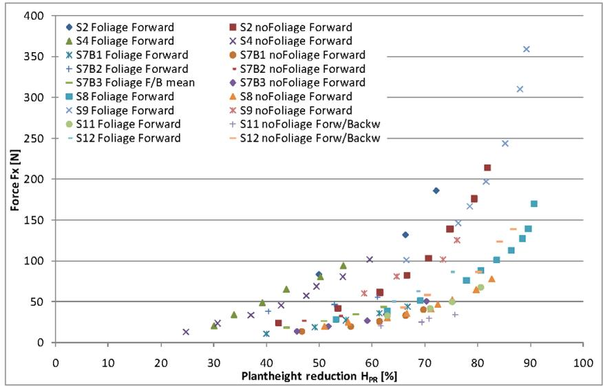
Fig. 22: Percental height reduction  $H_{PR}$  versus Force  $F_x$  of the tested willows
