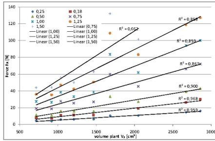
Fig. 25: Correlation between Force  $F_x$  and plant volume  $V_p$  at different velocities
