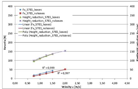
Fig. 16: Correlation between  $u$ ,  $F_x$  and  $H_{pr}$  for Salix 7 branch 3 in leafy and defoliated condition
