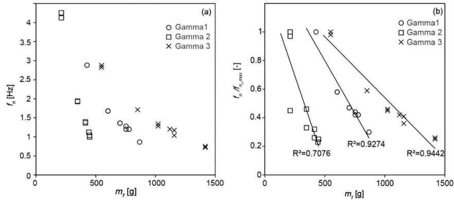
Fig. 6. Scatterplot of the relationship between the natural frequency  $f_n$  (a) and the normalised natural frequency  $f_n/f_{n,max}$  (b) with the fresh biomass  $m_f$  of the three specimens at different pruning phases (all axes with leaves-main stem).
