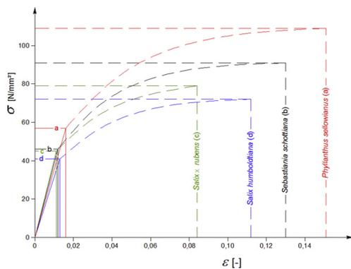
Fig. 3. Average trend stress/strain curves up to proportional limit (solid line) and further to ultimate load (dashed line) for the four species.
