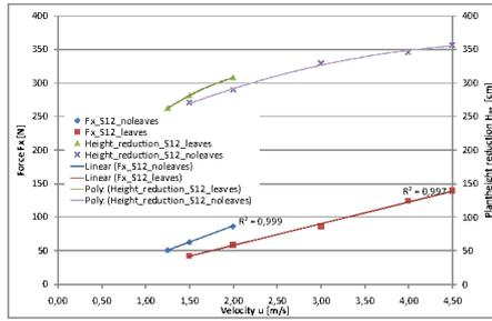
Fig. 20: Correlation between  $u$ ,  $F_x$  and  $H_{PR}$  for Salix 12 in leafy and defoliated condition
