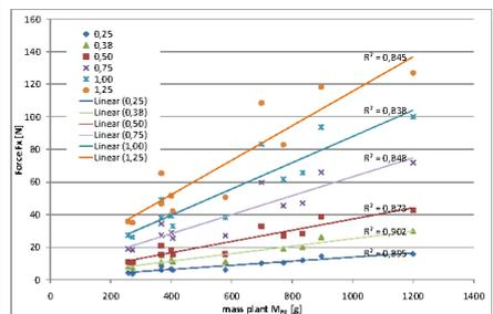
Fig. 24: Correlation between Force  $F_x$  no foliage and dry wood mass  $M_{Wpd}$  at different velocities
