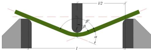
Fig. 1. Bending diagram, indicating the variables used in calculating the angle of inflection ( $\alpha$ ).
