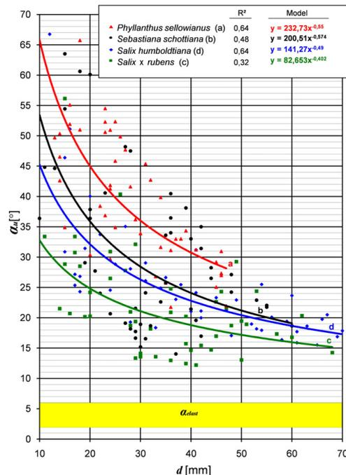
Fig. 4. Relationship between the diameter ( $d$ ) and the angle of inflection at failure ( $\alpha_u$ ). The band at the bottom of the graph shows the area of distribution of the angles of inflection at the proportional limit ( $\alpha_{elast}$ ).
