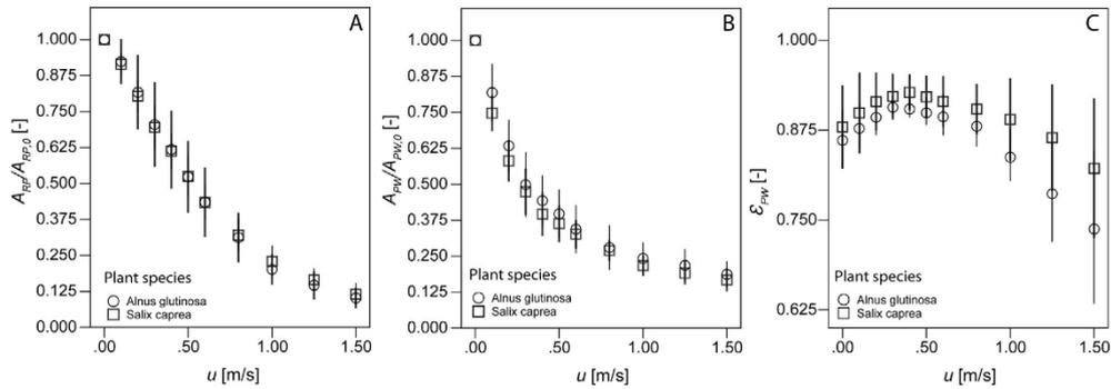
**Fig. 10.** The species averaged rectangular cross-sectional area occupied by the plant  $A_{RP}/A_{RP,0}$  (A), underwater frontal projected area  $A_{PW}/A_{PW,0}$  (B) and the underwater porosity of the plants  $\epsilon_{PW}$  (C) as a function of the velocity in foliated conditions. Note the different scaling for Y-axis in (C). Error bars show  $\pm 1$  standard error.
