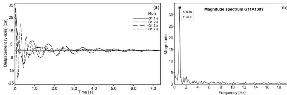
Fig. 5. Time history of the displacement of the main stem on the y-axis for Gamma 1 for different pruning stages, at a height of 130 cm (G1.1.a: all axes with leaves, G1.2.a: all axes without leaves, G1.3.a: axes 1–4 and G1.7.a only main stem), during pull and release tests (a). For reasons of readability, intermediate steps have been omitted. Spectral analyses for G1 in fully leaved condition (b).
