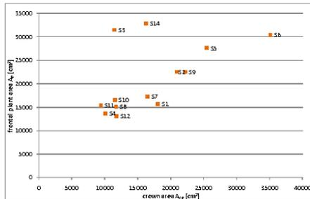
Fig. 11: Correlation between frontal projected area  $A_p$  and projected crown area  $A_{CP}$
