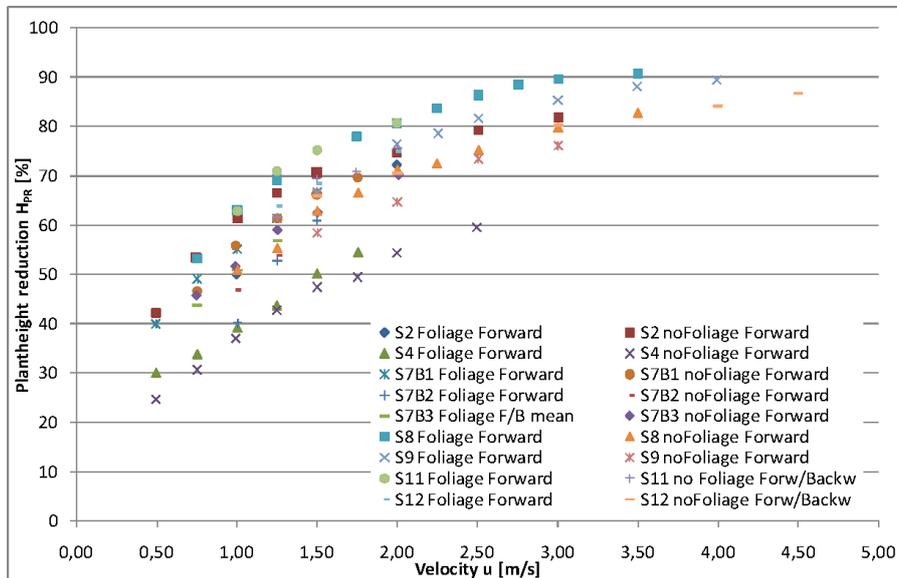
Fig. 21: Velocity  $u$  versus percental height reduction  $H_{PR}$  of the tested willows
