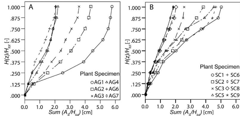
Fig. 7. Cumulative one-sided stem area over height of the investigated specimens of (A) *A. glutinosa* and (B) *S. caprea*.
