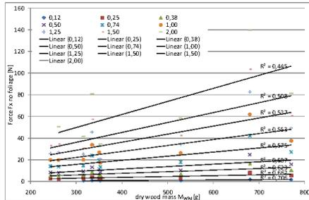
Fig. 23: Correlation between Force  $F_x$  and dry plant mass  $M_{pd}$  at different velocities
