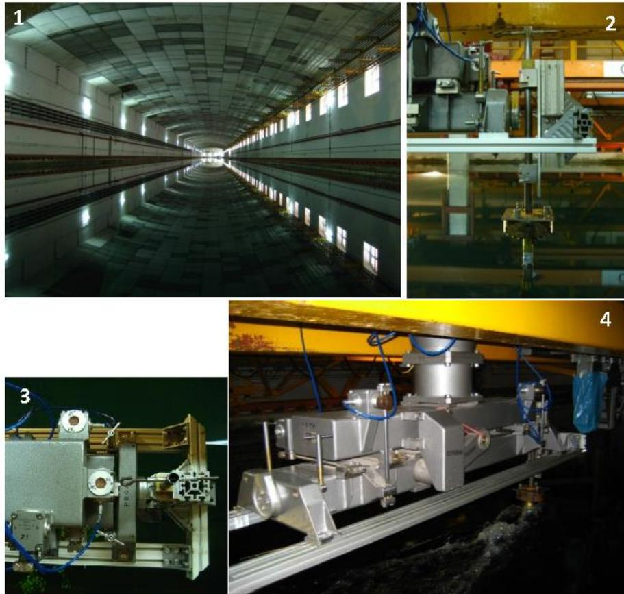
Fig. 1: Testing basin at El Pardo (1), side (2) and plane (3) view of the mounting device and carriage pulling plant through the channel (4)
