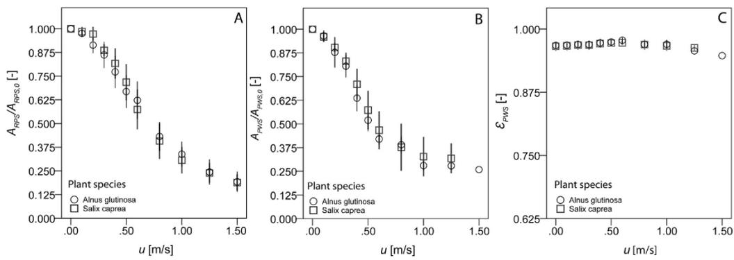
**Fig. 11.** Species-averaged rectangular cross-sectional area occupied by the plant  $A_{RPS}/A_{RPS,0}$  (A), underwater frontal projected area ( $A_{PWS}/A_{PWS,0}$ ) (B) and the porosity of the plants under water  $\epsilon_{PWS}$  (C) as a function of the velocity in defoliated conditions. Note the different scaling for Y-axis in (C). Error bars show  $\pm 1$  standard error.
