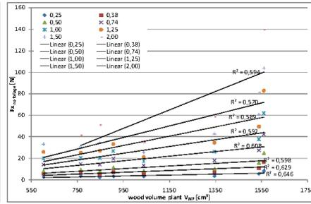
Fig. 26: Correlation between Force  $F_x$  and wood volume  $V_{wp}$  at different velocities
