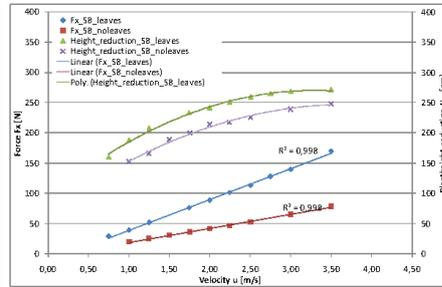
Fig. 17: Correlation between  $u$ ,  $F_x$  and  $H_{pr}$  for Salix 8 in leafy and defoliated condition
