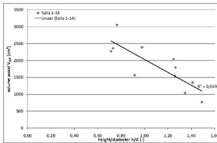
Fig. 4: Relation between displacement volume wood and height to diameter
