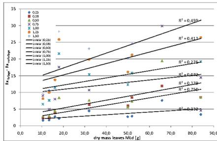
Fig. 27: Correlation between the differences of the forces between the runs with and without leaves and the dry leaf mass
