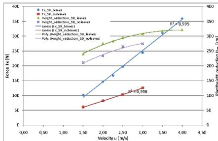
Fig. 18: Correlation between  $u$ ,  $F_x$  and  $H_{pr}$  for Salix 9 in leafy and defoliated condition
