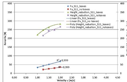
Fig. 19: Correlation between  $u$ ,  $F_x$  and  $H_{pr}$  for Salix 11 in leafy and defoliated condition
