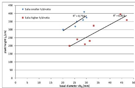
Fig. 3: Relation between plant height and basal diameter of the tested willows
