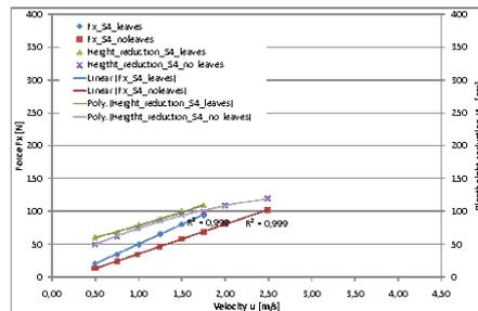
Fig. 13: Correlation between  $u$ ,  $F_x$  and  $H_{PR}$  for Salix 4 in leafy and defoliated condition
