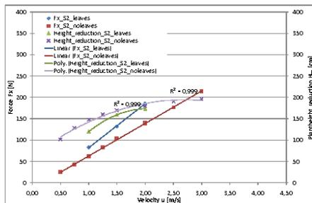
Fig. 12: Correlation between  $u$ ,  $F_x$  and  $H_{PR}$  for Salix 2 in leafy and defoliated condition
